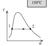
**4-45** A saturated water mixture contained in a spring-loaded piston-cylinder device is heated until the pressure and volume rise to specified values. The heat transfer and the work done are to be determined.
