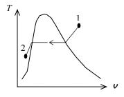
**4-38E** A cylinder contains water initially at a specified state. The water is heated at constant pressure. The final temperature of the water is to be determined, and the process is to be shown on a *T-v* diagram.
