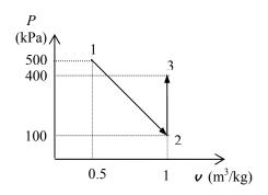
**4-7E** The boundary work done during the process shown in the figure is to be determined.
