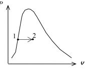
**4-40** [Also solved by EES on enclosed CD] A cylinder equipped with an external spring is initially filled with steam at a specified state. Heat is transferred to the steam, and both the temperature and pressure rise. The final temperature, the boundary work done by the steam, and the amount of heat transfer are to be determined, and the process is to be shown on a *P-v* diagram.
