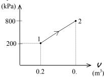
**4-128** A cylinder equipped with a set of stops for the piston is initially filled with saturated liquid-vapor mixture of water a specified pressure. Heat is transferred to the water until the volume increases by 20%. The initial and final temperature, the mass of the liquid when the piston starts moving, and the work done during the process are to be determined, and the process is to be shown on a *P-v* diagram.
