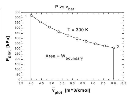
**4-22** CO<sub>2</sub> gas in a cylinder is compressed until the volume drops to a specified value. The pressure changes during the process with volume as  $P = a V^{-2}$ . The boundary work done during this process is to be determined.
