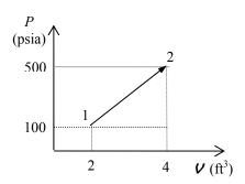
**4-8** A piston-cylinder device contains nitrogen gas at a specified state. The boundary work is to be determined for the polytropic expansion of nitrogen.
