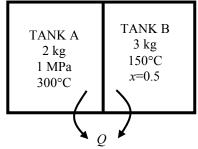
$$E_{\text{in}} - E_{\text{out}} = \Delta E_{\text{system}}$$
