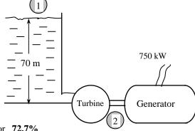
$$\eta_{\text{turbine-gen}} = \frac{\dot{W}_{\text{elect,out}}}{|\Delta \dot{E}_{\text{mech,fluid}}|} = \frac{750 \text{ kW}}{1031 \text{ kW}} = 0.727 \text{ or } 72.7\%$$
