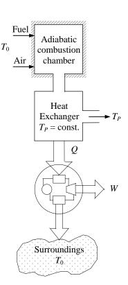
15-126 It is to be shown that the work output of the reversible heat engine operating at the specified
