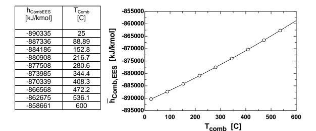
**15-50** The enthalpy of combustion of gaseous ethane at a 25°C and 1 atm is to be determined using the data from Table A-26 and to be compared to the value listed in Table A-27.
