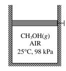
$$\overline{h}_{CO_2} + 2\overline{h}_{H_2O} + 5.64\overline{h}_{N_2} - 71.833 \times T_P = (1)(152,908) + (2)(127,952) + (5.64)(95,859) - (71.833)(2850) = 744,733 \text{ kJ} \text{ (Higher than 734,388 kJ)}$$
