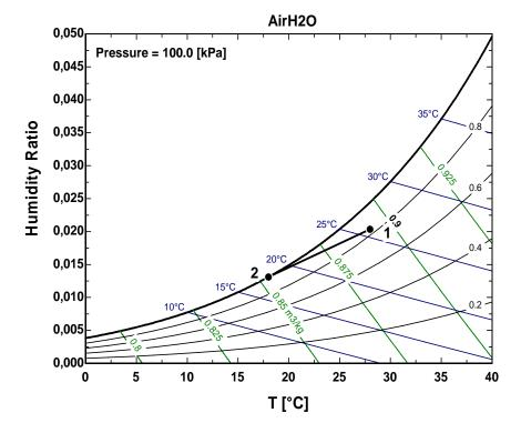
**14-94** An automobile air conditioner using refrigerant 134a as the cooling fluid is considered. The inlet and exit states of moist air in the evaporator are specified. The volume flow rate of the air entering the evaporator of the air conditioner is to be determined.
