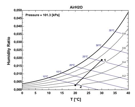
14-149 An uninsulated tank contains moist air at a specified state. Water is sprayed into the tank until the relative humidity in the tank reaches a certain value. The amount of water supplied to the tank, the final pressure in the tank, and the heat transfer during the process are to be determined.
