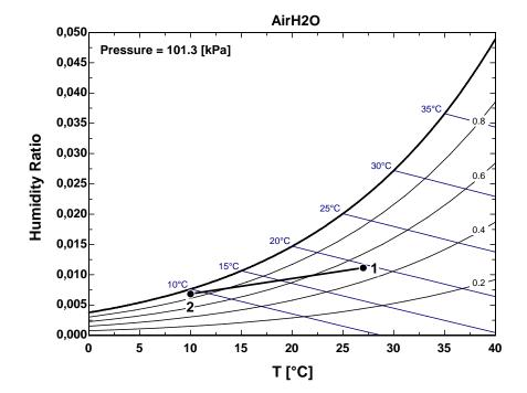
**14-93** Atmospheric air flows into an air conditioner that uses chilled water as the cooling fluid. The mass flow rate of the condensate water and the volume flow rate of chilled water supplied to the air conditioner are to be determined.
