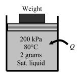
**12-29** A substance is heated in a piston-cylinder device until it turns from saturated liquid to saturated vapor at a constant pressure and temperature. The saturation pressure of this substance at a different temperature is to be estimated.
