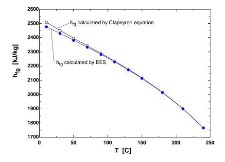
**12-28** A substance is heated in a piston-cylinder device until it turns from saturated liquid to saturated vapor at a constant pressure and temperature. The boiling temperature of this substance at a different pressure is to be estimated.
