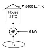
**6-97** A heat pump maintains a house at a specified temperature in winter. The maximum COPs of the heat pump for different outdoor temperatures are to be determined.
