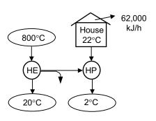
**6-132** A Carnot heat pump cycle is executed in a steady-flow system with R-134a flowing at a specified rate. The net power input and the ratio of the maximum-to-minimum temperatures are given. The ratio of the maximum to minimum pressures is to be determined.
