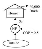
**6-50** The rate of heat loss from a house and the COP of the heat pump are given. The power consumption of the heat pump when it is running is to be determined.
