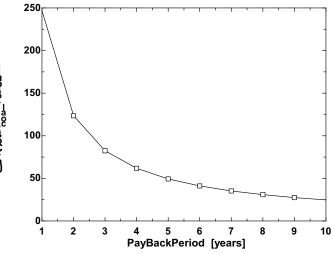
**6-26** The projected power needs of the United States is to be met by building inexpensive but inefficient coal plants or by building expensive but efficient IGCC plants. The price of coal that will enable the IGCC plants to recover their cost difference from fuel savings in 3 years is to be determined.
