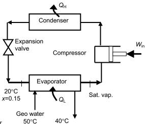
**Analysis** (a) The rate of heat transferred from the water is the energy change of the water from inlet to exit
