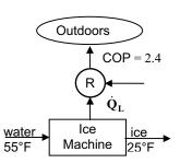
**6-43** The COP and the power consumption of a refrigerator are given. The time it will take to cool 5 watermelons is to be determined.
