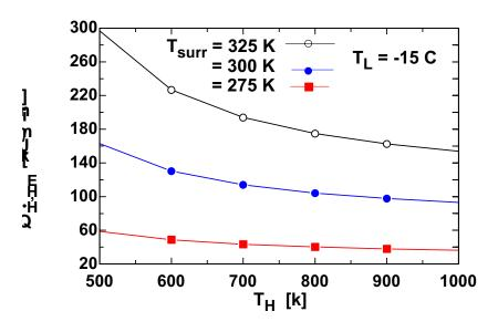
**6-130** Half of the work output of a Carnot heat engine is used to drive a Carnot heat pump that is heating a house. The minimum rate of heat supply to the heat engine is to be determined.
