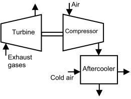
$$\dot{W}_{\rm T} = \dot{m}_{\rm exh} c_{p,\rm exh} (T_{\rm exh,1} - T_{\rm exh,2}) = (0.02 \text{ kg/s})(1.063 \text{ kJ/kg} \cdot \text{K})(400 - 350)\text{K} = 1.063 \text{ kW}$$
