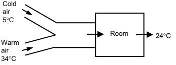
*Analysis* (*a*) We take the mixing chamber as the system, which is a control volume since mass crosses the boundary. The mass and energy balances for this steady-flow system can be expressed in the rate form as Mass balance:
