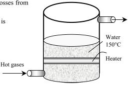
5-156 Cold water enters a steam generator at 20°C, and leaves as saturated vapor at  $T_{sat} = 150$ °C. The fraction of heat used to preheat the liquid water from 20°C to saturation temperature of 150°C is to be determined.
