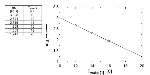
**5-88** Water is heated in a heat exchanger by geothermal water. The rate of heat transfer to the water and the exit temperature of the geothermal water is to be determined.
