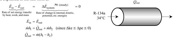
where at the inlet state  $h_1 = h_g = 268.57$  kJ/kg. Then the rates of
