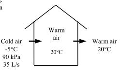
Then the sensible infiltration heat load corresponding to an infiltration rate of 35 L/s becomes
