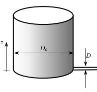
**5-146** The rate of accumulation of water in a pool and the rate of discharge are given. The rate supply of water to the pool is to be determined.
