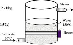
**5-157** Cold water enters a steam generator at 20°C and is boiled, and leaves as saturated vapor at boiler pressure. The boiler pressure at which the amount of heat needed to preheat the water to saturation temperature that is equal to the heat of vaporization is to be determined.
