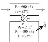
**5-128** A rigid tank initially contains saturated R-134a liquid-vapor mixture. The tank is connected to a supply line, and R-134a is allowed to enter the tank. The final temperature in the tank, the mass of R-134a that entered, and the heat transfer are to be determined.
