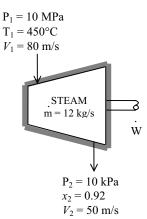
(b) There is only one inlet and one exit, and thus  $\dot{m}_1 = \dot{m}_2 = \dot{m}$ . We take the turbine as the system, which is a control volume since mass crosses the boundary. The energy balance for this steady-flow system can be expressed in the rate form as
