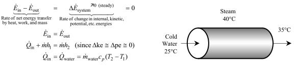
Then the rate of heat transfer to the water and the rate of condensation become
