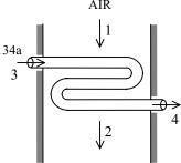
We take the entire heat exchanger as the system, which is a control volume. The mass and energy balances for this steady-flow system can be expressed in the rate form as
