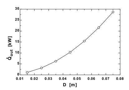
**5-112** A room is to be heated by an electric resistance heater placed in a duct in the room. The power rating of the electric heater and the temperature rise of air as it passes through the heater are to be determined.
