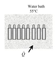
**5-171** Glass bottles are washed in hot water in an uncovered rectangular glass washing bath. The rates of heat and water mass that need to be supplied to the water are to be determined.
