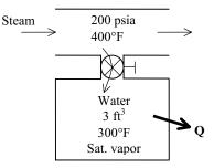
Analysis We take the tank as the system, which is a control volume since mass crosses the boundary. Noting that the microscopic energies of flowing and nonflowing fluids are represented by enthalpy h and internal energy u, respectively, the mass and energy balances for this uniform-flow system can be expressed as
