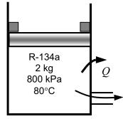
*Analysis* (a) We take the tank as the system, which is a control volume since mass crosses the boundary. Noting that the microscopic energies of flowing and nonflowing fluids are represented by enthalpy h and internal energy u, respectively, the mass and energy balances for this uniform-flow system can be expressed as
