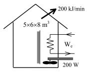
5-113 A house is heated by an electric resistance heater placed in a duct. The power rating of the electric heater is to be determined.
