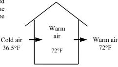
The reduction in the infiltration rate is 2.2 - 1.1 = 1.1 ACH. The reduction in the sensible infiltration heat load corresponding to it is
