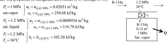
Analysis We take the tank as the system, which is a control volume since mass crosses the boundary. Noting that the microscopic energies of flowing and nonflowing fluids are represented by enthalpy h and internal energy u, respectively, the mass and energy balances for this uniform-flow system can be expressed as
