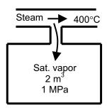
**5-144** Steam at a specified state is allowed to enter a piston-cylinder device in which steam undergoes a constant pressure expansion process. The amount of mass that enters and the amount of heat transfer are to be determined.
