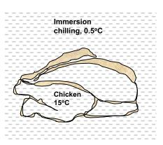
**5-166** Chickens are to be cooled by chilled water in an immersion chiller. The rate of heat removal from the chicken and the mass flow rate of water are to be determined.
