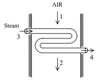
*Analysis* We take the entire heat exchanger as the system, which is a control volume. The mass and energy balances for this steady-flow system can be expressed in the rate form as
