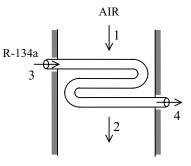
We take the entire heat exchanger as the system, which is a control volume. The mass and energy balances for this steady-flow system can be expressed in the rate form as
