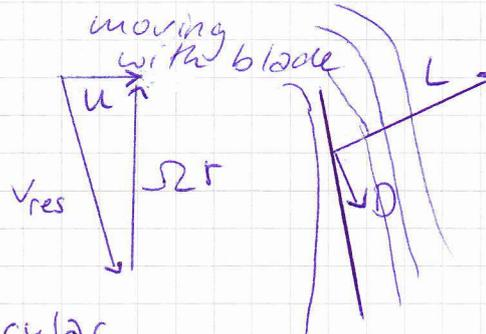
$\Omega r$  - speed component perpendicular to the wind →  $r$ : radius (c of rotor)
