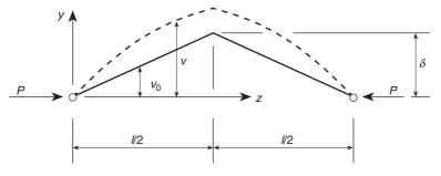
In this case, since each half of the column is straight before the application of P,  $d^2v_0/dz^2 = 0$  and Eq. (i) reduces to
