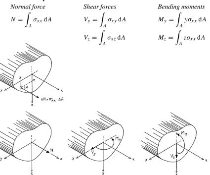
Positive directions of N,  $V_z$  and  $M_z$ The figure below shows the positive direction
