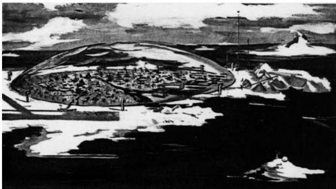
Figure 7.9 A spherical pneu designed by Frei Otto to cover a settlement in Antarctica.
