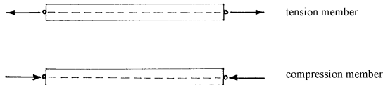
Figure 3.34 Two-force members are straight bars that can transfer forces only along their so-called bar axes.
