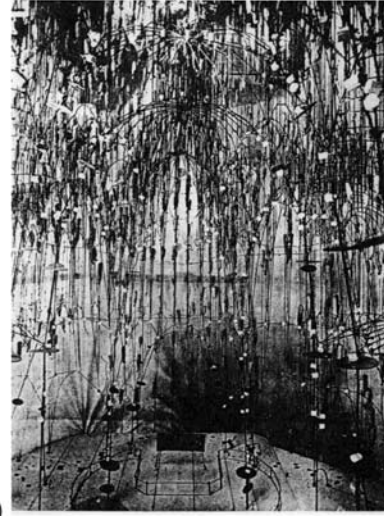
Figure 14.78 (b) Photograph of the inside of the model, rotated through 180^\circ . The upside-down cables change into arches. (c) Interior sketch by Gaudi on the basis of the model.
