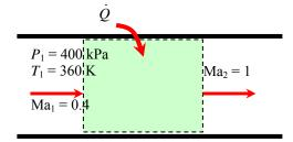
$$T_{01} = T_1 \left( 1 + \frac{k-1}{2} \text{ Ma}_1^2 \right) = (360 \text{ K}) \left( 1 + \frac{1.667 - 1}{2} 0.4^2 \right) = 379.2 \text{ K}$$
