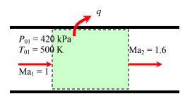
Then the exit stagnation temperature and heat transfer are determined to be
