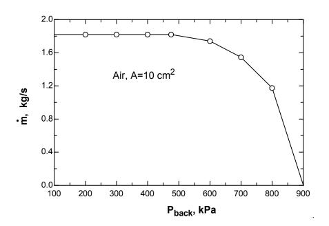
17-70E Air enters a converging-diverging nozzle at a specified temperature and pressure with low velocity. The pressure, temperature, velocity, and mass flow rate are to be calculated in the specified test section.
