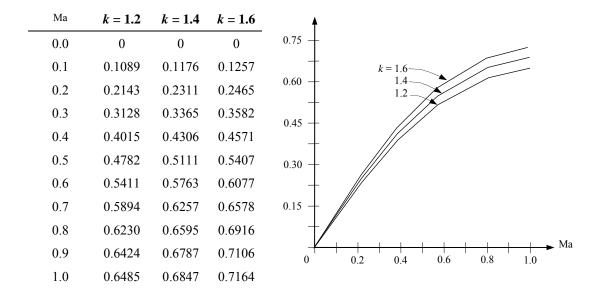
**Discussion** Note that the mass flow rate increases with increasing Mach number and specific heat ratio. It levels off at Ma = 1, and remains constant (choked flow).
