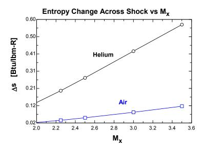
**17-89** Air flowing through a nozzle experiences a normal shock. Various properties are to be calculated before and after the shock.
