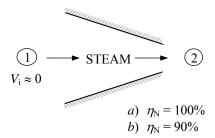
Then the exit velocity is determined from the steady-flow energy balance  $\dot{E}_{\rm in} = \dot{E}_{\rm out}$  with q = w = 0,
