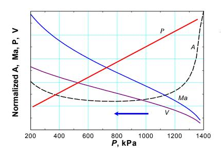
**17-60** For supersonic flow at the inlet, the variation of pressure, velocity, and Mach number along the length of the nozzle are to be sketched for an ideal gas under specified conditions.
