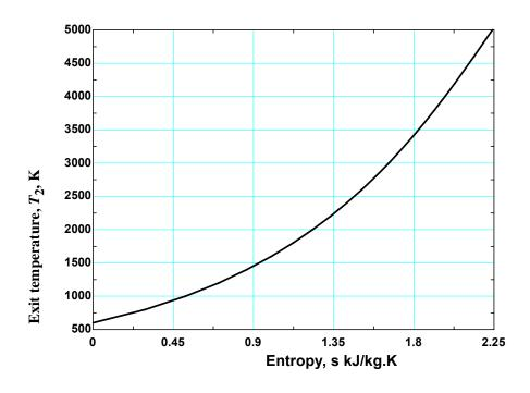
**17-111E** Air flowing with a subsonic velocity in a square duct is accelerated by heating until the flow is choked at the exit. The rate of heat transfer and the entropy change are to be determined.
