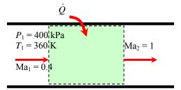
$$T_{01} = T_1 \left( 1 + \frac{k-1}{2} \text{ Ma}_1^2 \right) = (360 \text{ K}) \left( 1 + \frac{1.4-1}{2} 0.4^2 \right) = 371.5 \text{ K}$$
