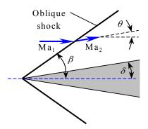
**17-93** Air flowing at a specified supersonic Mach number impinges on a two-dimensional wedge, The shock angle, Mach number, and pressure downstream of the weak and strong oblique shock formed by a wedge are to be determined.
