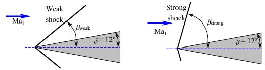
**Assumptions** 1 The flow is steady. 2 The boundary layer on the wedge is very thin. 3 Air is an ideal gas with constant specific heats.
