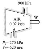
$$\dot{W}_{\rm in} = \dot{m}c_p (T_{02} - T_{01}) = (0.02 \text{ kg/s})(1.005 \text{ kJ/kg} \cdot \text{K})(562.4 - 300.2)\text{K} = 5.27 \text{ kW}$$
