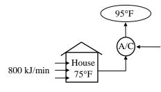
$$\dot{W}_{\text{net,in,min}} = \frac{\dot{Q}_L}{\text{COP}_{R,\text{max}}} = \frac{900 \text{ Btu/min}}{26.75} = 33.6 \text{ Btu/min} = \mathbf{0.79 \text{ hp}}$$
