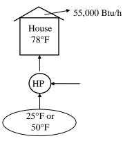
$$COP_{HP,max} = COP_{HP,rev} = \frac{1}{1 - (T_L / T_H)} = \frac{1}{1 - (50 + 460 \text{ R})/(78 + 460 \text{ R})} = 19.2$$
