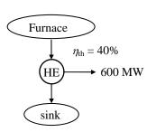
**6-18** The heat input and thermal efficiency of a heat engine are given. The work output of the heat engine is to be determined.
