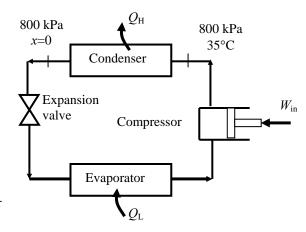
$$\dot{Q}_H = \dot{m}(h_1 - h_2) = (0.018 \text{ kg/s})(271.22 - 95.47) \text{ kJ/kg} = 3.164 \text{ kW}$$
