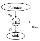
**6-22** The power output and fuel consumption rate of a power plant are given. The thermal efficiency is to be determined.
