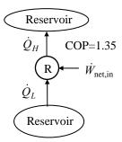
**6-44** The cooling effect and the COP of a refrigerator are given. The power input to the refrigerator is to be determined.
