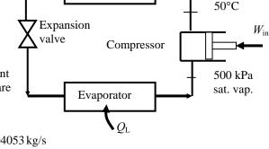
$$\dot{m}_R = \frac{\dot{V}_1}{v_1} = \frac{100 \text{ L/min} \left(\frac{1 \text{ m}^3}{1000 \text{ L}}\right) \left(\frac{1 \text{ min}}{60 \text{ s}}\right)}{0.04112 \text{ m}^3/\text{kg}} = 0.04053 \text{ kg/s}$$
