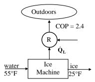
**6-47** The COP and the power consumption of a refrigerator are given. The time it will take to cool 5 watermelons is to be determined.
