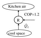
**6-41E** The heat absorption, the heat rejection, and the power input of a commercial heat pump are given. The COP of the heat pump is to be determined.
