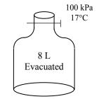
**5-123** An insulated rigid tank is evacuated. A valve is opened, and air is allowed to fill the tank until mechanical equilibrium is established. The final temperature in the tank is to be determined.
