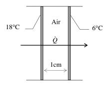
**2-114** Two surfaces of a flat plate are maintained at specified temperatures, and the rate of heat transfer through the plate is measured. The thermal conductivity of the plate material is to be determined.
