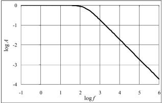
104. (*a*) The output voltage is the voltage across the resistor, which is the current through the circuit multiplied by the resistance. We calculate the current by dividing the input voltage by the impedance. Finally, we divide the output voltage by the input voltage to calculate the gain.
