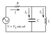
We combine these equations to eliminate the charge in the capacitor and the current in the inductor to write a single differential equation in terms of the current through the resistor.
