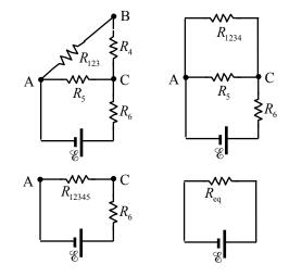
Resistors in series have the same current as their equivalent resistance, and resistors in parallel have the
