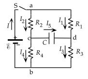
Use these currents to find the voltage at points c and d, which will give the voltage across the capacitor.
