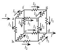
41. (a) To find the equivalent resistance between points a and c, apply a voltage between points a and c, find the current that flows from the voltage source, and then calculate
