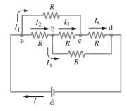
We have six unknown currents and six equations. We solve these equations by substitution. First, insert Eq. [3] into [6] to eliminate current  $I_5$ . Next insert Eq. [2] into Eqs. [1], [4], and [5] to eliminate  $I_2$ .
