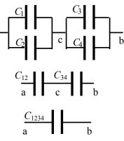
(b) The charge on the equivalent capacitor  $C_{1234}$  is given by  $Q_{1234} = C_{1234}V$ . This is the charge on both of the series components of  $C_{1234}$ . Note that  $V_{12} + V_{34} = V$ .
