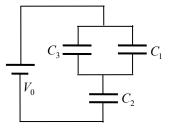
voltage drop across  $C_2$ , and then that voltage is subtracted from the battery voltage to find the voltage across the parallel combination.
