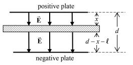
two original plates, and the new capacitance. Let x be the distance from one original plate to the nearest face of the sheet, and so  $d - \ell - x$  is the distance from the other original plate to the other face of the sheet.
