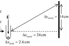
electron's motion, and see the diagram, which is a top view. First, during the horizontal acceleration phase, energy will be conserved and so the horizontal speed of the electron  $v_x$  can
