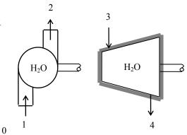
**7-117 EES** Problem 7-116 is reconsidered. The effect of the quality of the steam at the turbine exit on the net work output is to be investigated as the quality is varied from 0.5 to 1.0, and the net work output us to be plotted as a function of this quality.
