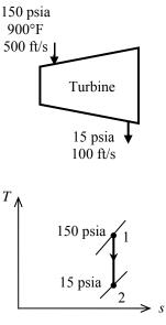
The exit temperature of the air for this isentropic process is
