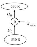
**7-29** A reversible heat pump with specified reservoir temperatures is considered. The entropy change of two reservoirs is to be calculated and it is to be determined if this heat pump satisfies the increase in entropy principle.
