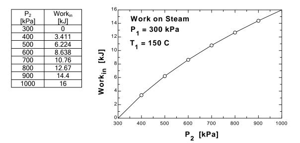
**7-49** A cylinder is initially filled with saturated water vapor at a specified temperature. Heat is transferred to the steam, and it expands in a reversible and isothermal manner until the pressure drops to a specified value. The heat transfer and the work output for this process are to be determined.
