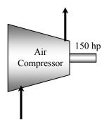
**7-181** The compressor of a facility is being cooled by air in a heat-exchanger. This air is to be used to heat the facility in winter. The amount of money that will be saved by diverting the compressor waste heat into the facility during the heating season is to be determined.
