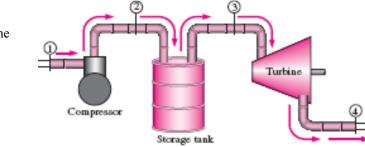
**7-220E** A system consisting of a compressor, a storage tank, and a turbine as shown in the figure is considered. The total work produced by the turbine and the total heat added to the air in the tank during the discharge are to be determined.
