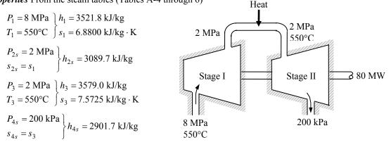
*Analysis* The power output of the actual turbine is given to be 80 MW. Then the power output for the isentropic operation becomes
