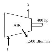
Analysis (a) We take the compressor as the system, which is a control volume since mass crosses the boundary. The energy balance for this
