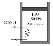
We take the contents of the cylinder as the system. This is a closed system since no mass enters or leaves. The energy balance for this stationary closed system can be expressed as
