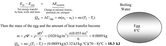
We again take a single egg as the system The entropy generated during this process can be determined by applying an entropy balance on an *extended system* that includes the egg and its immediate surroundings so that the boundary temperature of the extended system is at 97°C at all times:
