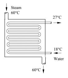
**7-148** Cold water is heated by hot water in a heat exchanger. The rate of heat transfer and the rate of entropy generation within the heat exchanger are to be determined.
