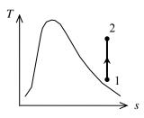
**7-38E** R-134a is expanded isentropically in a closed system. The heat transfer and work production are to be determined.
