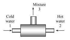
where the subscript 1 denotes the cold water stream, 2 the hot water stream, and 3 the mixture.
