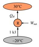
**7-185** The operating conditions and thermal reservoir temperatures of a heat pump are given. It is to be determined if the increase of entropy principle is satisfied.
