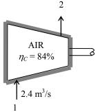
**7-138** Air is compressed by an adiabatic compressor from a specified state to another specified state. The isentropic efficiency of the compressor and the exit temperature of air for the isentropic case are to be determined.
