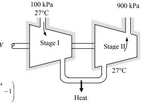
**7-207** A three-stage compressor with two stages of intercooling is considered. The two intermediate pressures that will minimize the work input are to be determined in terms of the inlet and exit pressures.
