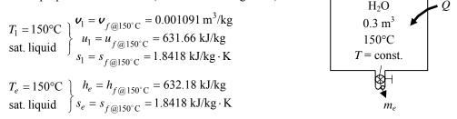
*Analysis* (*a*) We take the tank as the system, which is a control volume since mass crosses the boundary. Noting that the microscopic energies of flowing and nonflowing fluids are represented by enthalpy h and internal energy u, respectively, the mass and energy balances for this uniform-flow system can be expressed as
