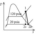
$$P_{2} = 20 \text{ psia} \\ s_{2s} = s_{1} \\ \begin{cases} x_{2s} = \frac{s_{2s} - s_{f}}{s_{fg}} = \frac{0.22362 - 0.02605}{0.19962} = 0.9897 \\ u_{2s} = u_{f} + x_{2s}u_{fg} = 11.401 + (0.9897)(82.898) = 93.445 \text{ Btu/lbm} \end{cases}$$
