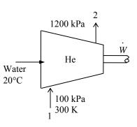
Sample Analysis: We take the compressor exit temperature to be  $T_2 = 200^{\circ}\text{C} = 473$  K. Then,
