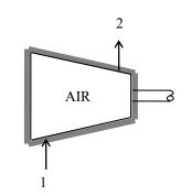
**7-139E** Argon enters an adiabatic compressor with an isentropic efficiency of 80% at a specified state, and leaves at a specified pressure. The exit temperature of argon and the work input to the compressor are to be determined.
