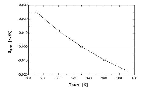
**7-42E** A cylinder is initially filled with R-134a at a specified state. The refrigerant is cooled and condensed at constant pressure. The entropy change of refrigerant during this process is to be determined
