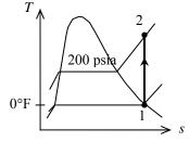
7-60 Steam is expanded in an isentropic turbine. The work produced is to be determined.
