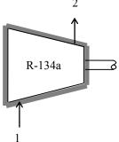
There is only one inlet and one exit, and thus  $\dot{m}_1 = \dot{m}_2 = \dot{m}$ . We take the compressor as the system, which is a control volume since mass crosses the boundary. The energy balance for this steady-flow system can be expressed in the rate form as
