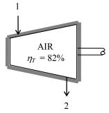
There is only one inlet and one exit, and thus  $\dot{m}_1 = \dot{m}_2 = \dot{m}$ . We take the actual turbine as the system, which is a control volume since mass crosses the boundary. The energy balance for this steady-flow system can be expressed as
