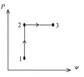
**4-85** [Also solved by EES on enclosed CD] A cylinder equipped with a set of stops on the top is initially filled with air at a specified state. Heat is transferred to the air until the piston hits the stops, and then the pressure doubles. The work done by the air and the amount of heat transfer are to be determined, and the process is to be shown on a *P-v* diagram.
