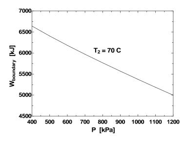
**4-14E** Superheated water vapor in a cylinder is cooled at constant pressure until 70% of it condenses. The boundary work done during this process is to be determined.
