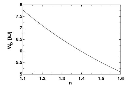
**4-19** Nitrogen gas in a cylinder is compressed polytropically until the temperature rises to a specified value. The boundary work done during this process is to be determined.
