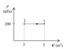
**4-6** The boundary work done during the process shown in the figure is to be determined.
