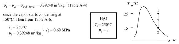
**3-63** Heat is supplied to a piston-cylinder device that contains water at a specified state. The volume of the tank, the final temperature and pressure, and the internal energy change of water are to be determined.
