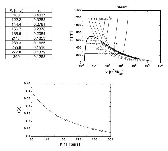
**3-58** A rigid vessel that contains a saturated liquid-vapor mixture is heated until it reaches the critical state. The mass of the liquid water and the volume occupied by the liquid at the initial state are to be determined.
