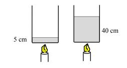
**3-50** A vertical piston-cylinder device is filled with water and covered with a 20-kg piston that serves as the lid. The boiling temperature of water is to be determined.
