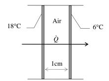
**2-114** Two surfaces of a flat plate are maintained at specified temperatures, and the rate of heat transfer through the plate is measured. The thermal conductivity of the plate material is to be determined.
