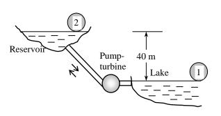
$$\dot{W}_{\text{max, turbine}} = \dot{W}_{\text{min, pump}} = \dot{W}_{\text{ideal}} = \Delta \dot{E}_{\text{mech}} = \dot{m} \Delta e_{\text{mech}} = \dot{m} \Delta p e = \dot{m} g \Delta z = \rho \dot{U}_g \Delta z$$
