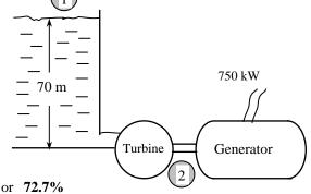
Therefore, the reservoir supplies 1031 kW of mechanical energy to the turbine, which converts 800 kW of it to shaft work that drives the generator, which generates 750 kW of electric power.
