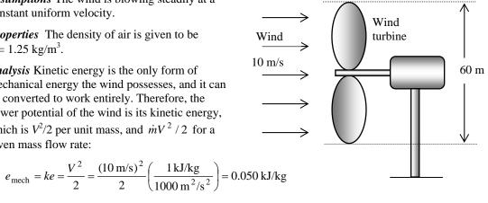
$$\dot{m} = \rho VA = \rho V \frac{\pi D^2}{4} = (1.25 \text{ kg/m}^3)(10 \text{ m/s}) \frac{\pi (60 \text{ m})^2}{4} = 35,340 \text{ kg/s}$$
