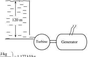
$$e_{\text{mech}} = pe = gz = (9.81 \text{ m/s}^2)(120 \text{ m}) \left(\frac{1 \text{ kJ/kg}}{1000 \text{ m}^2/\text{s}^2}\right) = 1.177 \text{ kJ/kg}$$
