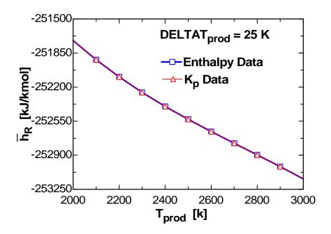
**16-107** The  $K_P$  value of the dissociation process  $O_2 \Leftrightarrow 2O$  at a specified temperature is to be determined using the  $\overline{h}_R$  data and  $K_P$  value at a specified temperature.
