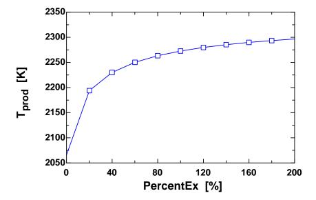
**16-33E** Carbon monoxide is burned with 100 percent excess air. The temperature at which 97 percent of CO burn to CO<sub>2</sub> is to be determined.
