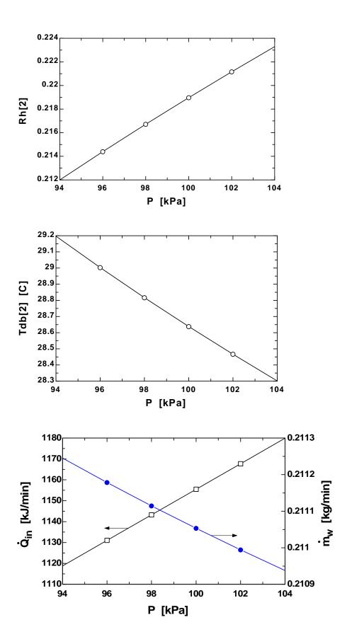
**14-145** Air is heated and dehumidified in an air-conditioning system consisting of a heating section and an evaporative cooler. The temperature and relative humidity of the air when it leaves the heating section, the rate of heat transfer in the heating section, and the rate at which water is added to the air in the evaporative cooler are to be determined.
