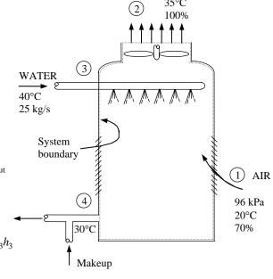
The properties of air at the inlet and the exit are
