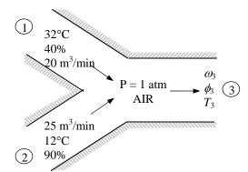
**14-108** Two airstreams are mixed steadily. The specific humidity, the relative humidity, the dry-bulb temperature, and the volume flow rate of the mixture are to be determined.
