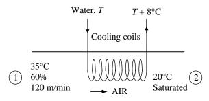
The amount of moisture in the air decreases due to dehumidification  $(\omega_2 < \omega_1)$ . The inlet and the exit states of the air are completely specified, and the total pressure is 95 kPa. Then the properties of the air at both states are determined to be
