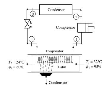
$$m_a = \frac{V_1}{V_1} = \frac{1000 \text{ m}^3}{0.905 \text{ m}^3 / \text{kg dry air}} = 1105 \text{ kg}$$
