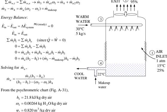
14-118 Water is cooled by air in a cooling tower. The exergy lost in the cooling tower is to be determined.
