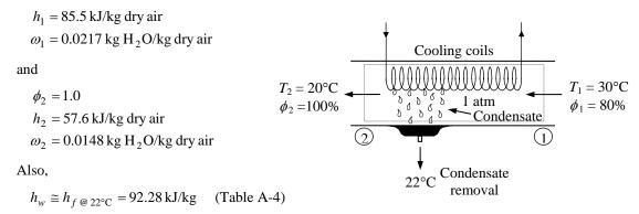
**Analysis** The amount of moisture in the air decreases due to dehumidification ( $\omega_2 < \omega_1$ ). Applying the water mass balance and energy balance equations to the combined cooling and dehumidification section,
