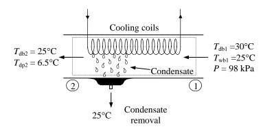
The partial pressure of water vapor at the exit state is
