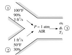
Analysis The mass flow rate of dry air in each stream is
