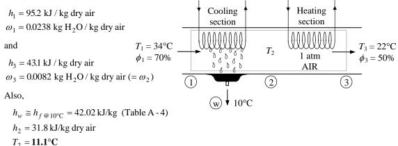
(b) The amount of heat removed in the cooling section is determined from the energy balance equation applied to the cooling section,
