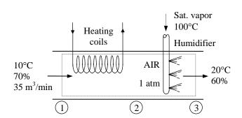
$$\dot{m}_a = \frac{\dot{V_1}}{v_1} = \frac{35 \text{ m}^3 / \text{min}}{0.809 \text{ m}^3 / \text{kg}} = 43.3 \text{ kg/min}$$
