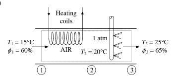
$$\Delta \omega = \omega_3 - \omega_2 = 0.0129 - 0.0064 = 0.0065 \text{ kg H}_2\text{O}/\text{kg dry air}$$
