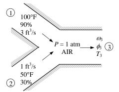
14-110E Two airstreams are mixed steadily. The rate of entropy generation is to be determined.
