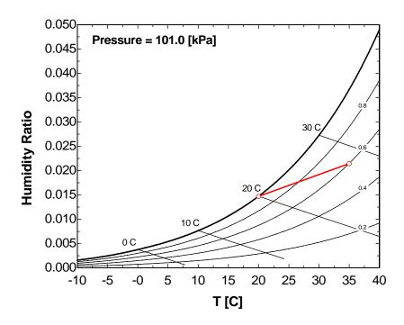
**14-86** Air is cooled by passing it over a cooling coil. The rate of heat transfer, the mass flow rate of water, and the exit velocity of airstream are to be determined.
