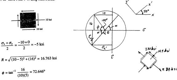
$\alpha = 100 - 72.646 = 27.354^{\circ}$   $\sigma_{x'} = -5 - 16.763 \cos 27.354^{\circ} = -19.9 \text{ ksi}$  Ans  $\tau_{x'y'} = 16.763 \sin 27.354^{\circ} = 7.70 \text{ ksi}$  Ans  $\sigma_{y'} = 16.763 \cos 27.354^{\circ} - 5 = 9.89 \text{ ksi}$
