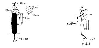
$+ \Sigma F_y = 0;$  12 cos 30° - N = 0; N = 10.392 kN  $+ \Sigma F_x = 0;$  -12 sin 30° + V = 0; V = 6 kN
