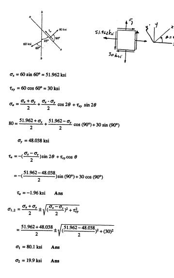
**9-21.** The stress acting on two planes at a point is indicated. Determine the normal stress  $\sigma_b$  and the principal stresses at the point.
