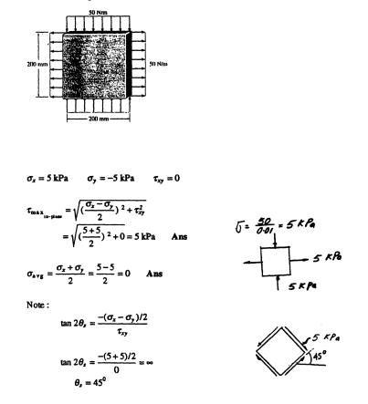
**9-27** The square steel plate has a thickness of 0.5 in. and is subjected to the edge loading shown. Determine the principal stresses developed in the steel.
