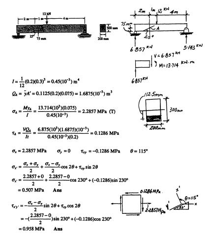
**9-23.** The wood beam is subjected to a distributed loading. Determine the principal stresses at point A and specify the orientation of the element.
