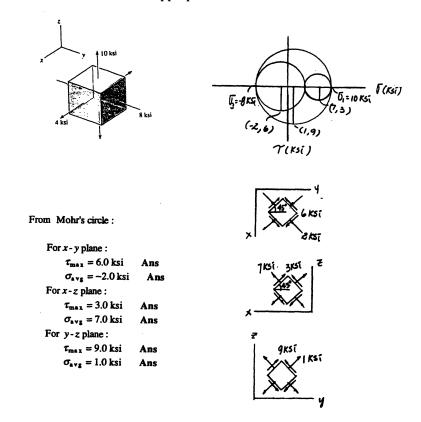
**9-91** The stress at a point is shown on the element. Determine the principal stresses and the absolute maximum shear stress.
