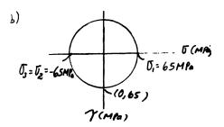
**9-90.** The principal stresses acting at a point in a body are shown. Draw the three Mohr's circles that describe this state of stress and find the maximum in-plane shear stresses and associated average normal stresses for the x-y, y-z, and x-z planes. For each case, show the results on the element oriented in the appropriate direction.
