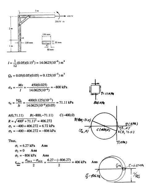
**9–98** The stress at a point is shown on the element. Determine the principal stresses and the absolute maximum shear stress.
