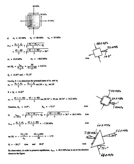
**\*9-104** The state of stress at a point in a member is shown on the element. Determine the stress components acting on the inclined plane AB. Solve the problem using the method of equilibrium described in Sec. 9.1.
