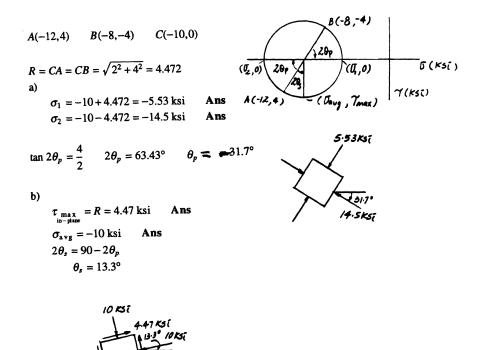
9-74 Determine (a) the principal stresses and (b) the maximum in-plane shear stress and average normal stress. Specify the orientation of the element in each case.
