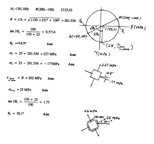
9-71 Determine (a) the principal stresses and (b) the maximum in-plane shear stress and average normal stress. Specify the orientation of the element in each case.
