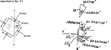
$$\begin{array}{l} + \Sigma F_{x'} = 0; \\ + 50\Delta A \sin 30^{\circ} \cos 60^{\circ} - 28\Delta A \cos 30^{\circ} \cos 60^{\circ} \\ + 50\Delta A \sin 30^{\circ} \cos 60^{\circ} - 28\Delta A \sin 30^{\circ} \cos 30^{\circ} = 0 \\ \Delta F_{x'} = - 33.251\Delta A \end{array}$$
