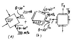
**9-19** The stress along two planes at a point is indicated. Determine the normal stresses on plane b-b and the principal stresses.
