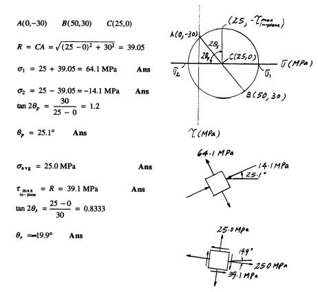
\*9-76. Determine (a) the principal stresses and (b) the maximum in-plane shear stress and average normal stress. Specify the orientation of the element in each case.
