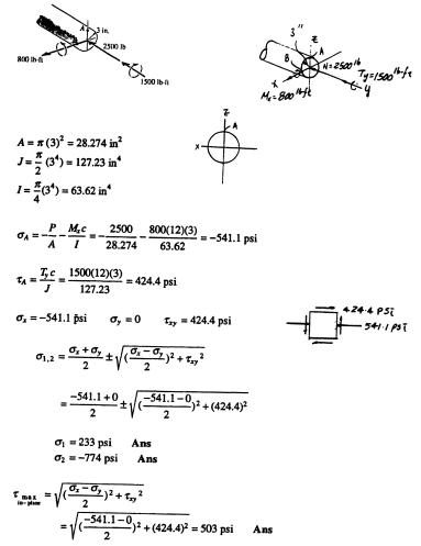
**9-47.** The internal loadings at a cross section through the 6-in.-diameter drive shaft of a turbine consist of an axial force of 2500 lb, a bending moment of 800 lb  $\cdot$  ft, and a torsional moment of 1500 lb  $\cdot$  ft. Determine the principal stresses at point *B*. Also calculate the maximum in-plane shear stress at this point.
