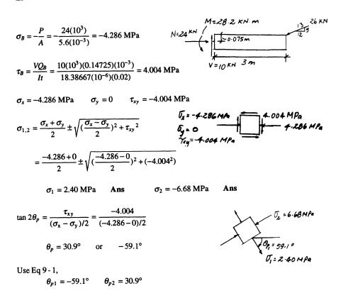
**9-39** The wide-flange beam is subjected to the 50-kN force. Determine the principal stresses in the beam at point A located on the *web* at the bottom of the upper flange. Although not very accurate, use the shear formula to compute the shear stress.
