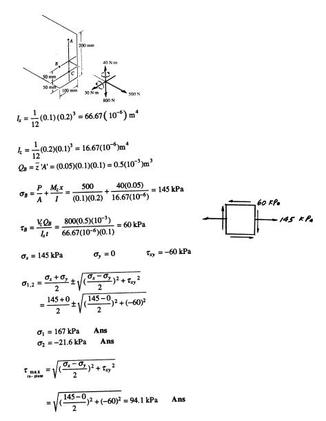
**9–53** The internal loadings at a section of the beam consist of an axial force of 500 N, a shear force of 800 N, and two moment components of 30 N  $\cdot$  m and 40 N  $\cdot$  m. Determine the principal stresses at point C. Also compute the maximum in-plane shear stress at this point.
