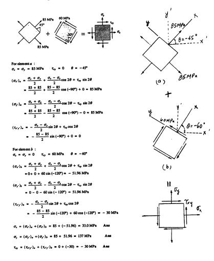
9-18 A point on a thin plate is subjected to the two successive states of stress shown. Determine the resultant state of stress represented on the element oriented as shown on the right.
