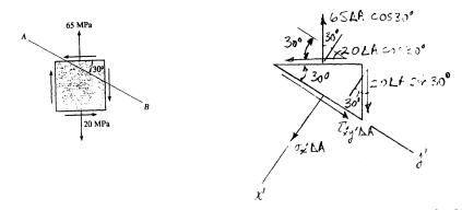
$4 \Sigma F_x = 0; \qquad \sigma_{x'} \Delta A + 20 \Delta A \sin 30^\circ \cos 30^\circ + 20 \Delta A \cos 30^\circ \cos 60^\circ - 65 \Delta A \cos 30^\circ \cos 30^\circ = 0$  $\sigma_{x'} = 31.4 \text{ MPa} \qquad \text{Ans}$
