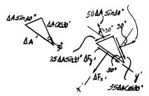
$\chi + \Sigma F_{y'} = 0$   $\Delta F_{y'} - 50 \Delta A \sin 30^{\circ} \cos 30^{\circ} - 35 \Delta A \sin 30^{\circ} \cos 60^{\circ} + 90 \Delta A \cos 30^{\circ} \sin 30^{\circ} + 35 \Delta A \cos 30^{\circ} \sin 60^{\circ} = 0$  $\Delta F_{y'} = -34.82 \Delta A$
