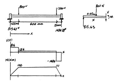
6-7 Draw the shear and moment diagrams for the beam.
