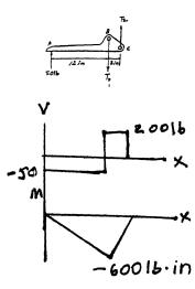
**6-3** Draw the shear and moment diagrams for the shaft. The bearings at A and D exert only vertical reactions on the shaft. The loading is applied to the pulleys at B and C and E.
