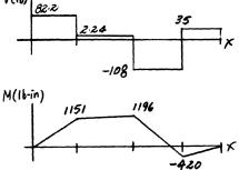
\*6-4 Draw the shear and moment diagrams for the beam.
