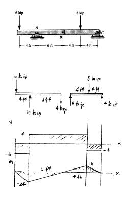
**6-13** The bars are connected by pins at C and D. Draw the shear and moment diagrams for the assembly. Neglect the effect of axial load.
