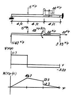
6-10. The engine crane is used to support the engine, which has a weight of 1200 lb. Draw the shear and moment diagrams of the boom ABC when it is in the horizont position shown.
