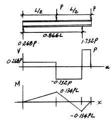
\*6-12 Draw the shear and moment diagrams for the compound beam which is pin connected at B.
