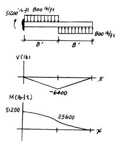
6-17 The 150-lb man sits in the center of the boat, which has a uniform width and a weight per linear foot of 3 lb/ft. Determine the maximum bending moment exerted on the boat. Assume that the water exerts a uniform distributed load upward on the bottom of the boat.
