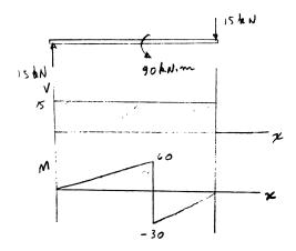
**6-6.** Draw the shear and moment diagrams for the shaft. The bearings at A and B exert only vertical reactions on the shaft. Also, express the shear and moment in the shaft as a function of x within the region 125 mm < x < 725 mm.
