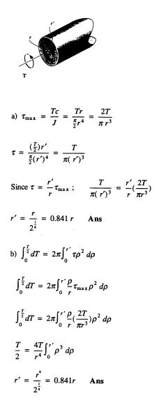
5-3. The solid shaft of radius r is subjected to a torque **T**. Determine the radius r' of the inner core of the shaft that resists one-quarter of the applied torque (T/4). Solve the problem two ways: (a) by using the torsion formula, (b) by finding the resultant of the shear-stress distribution.
