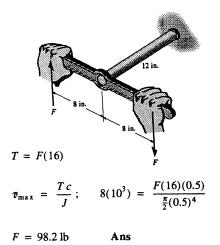
5-17 The steel shaft has a diameter of 1 in. and is screwed into the wall using a wrench. Determine the maximum shear stress in the shaft if the couple forces have a magnitude of F = 30 lb.
