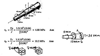
**5-19.** The steel shaft is subjected to the torsional loading shown. Determine the absolute maximum shear stress in the shaft and sketch the shear-stress distribution along a radial line where it is maximum.
