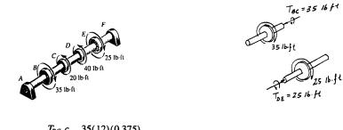
$$(\tau_{BC})_{\max} = \frac{T_{BC}}{J} = \frac{55(12)(0.575)}{\frac{\pi}{2}(0.375)^4} = 5070 \text{ psi} = 5.07 \text{ ksi}$$
