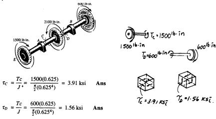
5-7. The shaft has an outer diameter of 1.25 in. and an inner diameter of 1 in. If it is subjected to the applied torques as shown, determine the absolute maximum shear stress developed in the shaft. The smooth bearings at A and B do not resist torque.
