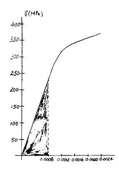
\*3-4 A tension test was performed on a steel specimen having an original diameter of 0.503 in. and gauge length of 2.00 in. The data is listed in the table. Plot the stress-strain diagram and determine approximately the modulus of elasticity, the yield stress, the ultimate stress, and the rupture stress. Use a scale of 1 in. = 20 ksi and 1 in. = 0.05 in./in. Redraw the elastic region, using the same stress scale but a strain scale of 1 in. = 0.001 in./in.
