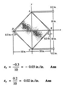
\*2-16 The corners of the square plate are given the displacements indicated. Determine the shear strain along the edges of the plate at A and B.
