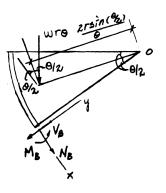
\*1-32. The curved rod AD of radius r has a weight per length of w. If it lies in the horizontal plane, determine the resultant internal loadings acting on the cross section through point B. Hint: The distance from the centroid C of segment AB to point O is CO = 0.9745r.
