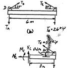
1-10 Determine the resultant internal loadings acting on the cross sections through points D and E of the frame.
