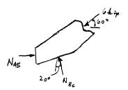
1-54 The two members used in the construction of an aircraft fuselage are joined together using a 30° fish-mouth weld. Determine the average normal and average shear stress on the plane of each weld. Assume each inclined plane supports a horizontal force of 400 lb.
