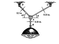
$$\sigma_{AD} = \frac{T_{AD}}{\frac{\pi}{4}(0.3)^2}; \qquad T_{AD} = (0.070686)\sigma_{AD}$$
