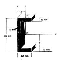
$$\bar{x} = \frac{\Sigma \bar{x}A}{\Sigma A} = \frac{(62.5)(2)(125)(15) + (7.5)(270)(15)}{2(125)(15) + 270(15)} = 33.942 \text{ mm} = 33.9 \text{ mm}$$
