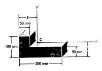
$$\bar{x} = \frac{\Sigma \bar{x}A}{\Sigma A} = \frac{25(50)(50) + 100(50)(200)}{50(50) + (50)(200)} = 85 \text{ mm}$$
