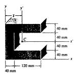
$$\bar{x} = \frac{\Sigma \tilde{x}A}{\Sigma A} = \frac{(20)(160)(40) + 2[100(120)(40)]}{160(40) + 2[120(40)]} = 68.0 \text{ mm}$$
