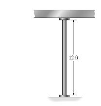
**13–19.** The 12-ft A-36 steel column has an outer diameter of 3 in. and a thickness of 0.25 in. Determine the critical load if the bottom is fixed and the top is pinned.
