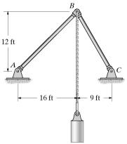
\*13-32. The linkage is made using two A-36 steel rods, each having a circular cross section. If each rod has a diameter of  $\frac{3}{4}$  in., determine the largest load it can support without causing any rod to buckle. Assume that the rods are pin connected at their ends.
