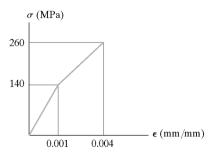
Tangent modulus: From the stress-strain diagram,
