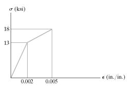
13–75. Construct the buckling curve, P/A versus L/r, for a column that has a bilinear stress-strain curve in compression as shown.
