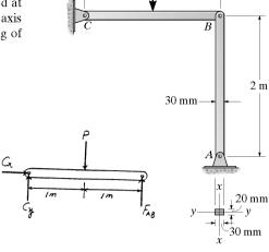
With respect to y - y axis, K = 0.5 (column with both ends fixed).
