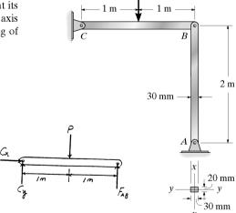
With respect to y - y axis, K = 0.5 (column with both ends fixed).
