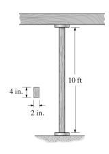
**13–21.** The 10-ft column has the dimensions shown. Determine the critical load if the bottom is fixed and the top is pinned.  $E_{\rm w}=1.6(10^3)$  ksi,  $\sigma_Y=5$  ksi.
