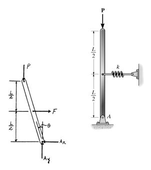
**13–2.** The column consists of a rigid member that is pinned at its bottom and attached to a spring at its top. If the spring is unstretched when the column is in the vertical position, determine the critical load that can be placed on the column.
