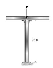
Critical Buckling Load:  $I_y = 88.6 \text{ in}^4 \text{ for a W8} \times 67 \text{ wide}$  flange section and K = 0.7 for one end fixed and the other end pinned. Applying Euler's formula,
