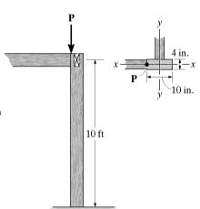
\*13–60. The wood column is fixed at its base and can be assumed fixed connected at its top. Determine the maximum eccentric load P that can be applied without causing the column to buckle or yield.  $E_{\rm w}=1.8(10^3)$  ksi,  $\sigma_Y=8$  ksi.
