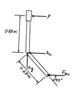
\*13–36. Determine the maximum allowable load P that can be applied to member BC without causing member AB to buckle. Assume that AB is made of steel and is pinned at its ends for x-x axis buckling and fixed at its ends for y-y axis buckling. Use a factor of safety with respect to buckling of F.S. = 3.  $E_{\rm st} = 200$  GPa,  $\sigma_Y = 360$  MPa.
