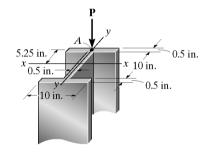
Interaction Formula: Bending is about x - x axis. Applying Eq. 13-31, we have
