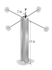
**13–67.** The W14  $\times$  53 structural A-36 steel column is fixed at its base and free at its top. If P=75 kip, determine the sidesway deflection at its top and the maximum stress in the column.
