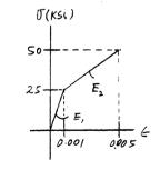
\*13–76. Construct the buckling curve, P/A versus L/r, for a column that has a bilinear stress–strain curve in compression as shown. The column is pinned at its ends.
