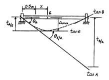
\*12–76. Determine the slope of the 20-mm-diameter A-36 steel shaft at the bearings at A and B. The bearings exert only vertical forces on the shaft.
