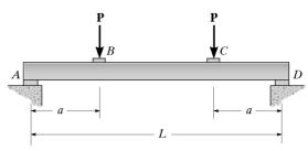
**Moment - Area** Theorems: Due to symmetry, the slope at midspan (point E) is zero. Hence the maximum displacement is,
