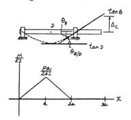
**12–139.** The W8  $\times$  24 simply supported beam is subjected to the loading shown. Using the method of superposition, determine the deflection at its center C. The beam is made of A-36 steel.
