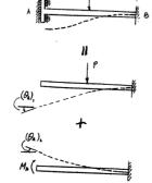
**12–127.** Determine the reactions at the supports A and B. EI is constant.
