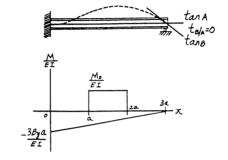
**12–119.** Determine the value of a for which the maximum positive moment has the same magnitude as the maximum negative moment. EI is constant.
