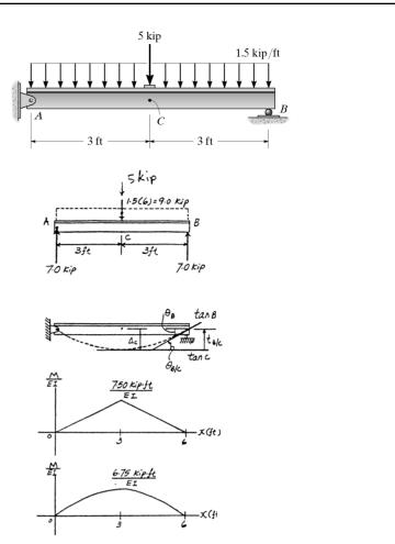
**12–89.** The W8  $\times$  48 cantilevered beam is made of A-36 steel and is subjected to the loading shown. Determine the displacement at its end A.
