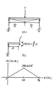
**12–14.** Determine the equation of the elastic curve for the beam using the x coordinate. Specify the slope at A and the maximum deflection. EI is constant.
