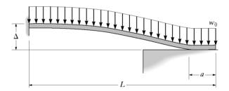
The curvature of the beam in region BC is zero, therefore there is no bending moment in the region BC. The reaction F is at B where it touches the support. The slope is zero at this point and the deflection is  $\Delta$  where
