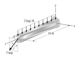
**Method of Superposition:** Using the table in Appendix C, the required vertical displacements are
