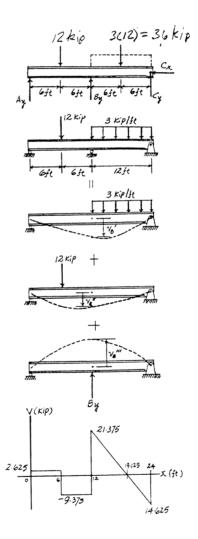
**12–125.** Determine the reactions at support C.EI is constant for both beams.
