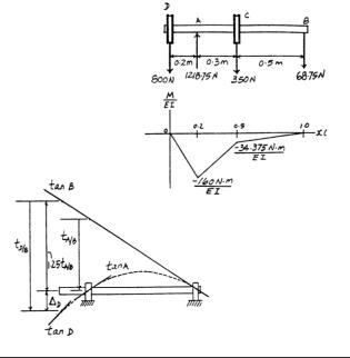
**12–78.** The beam is subjected to the loading shown. Determine the slope at B and deflection at C. EI is constant.
