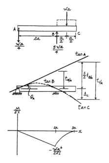
12-137. Determine the maximum deflection between the supports A and B. EI is constant. Use the method of integration.
