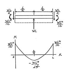
**12–142.** Determine the moment reactions at the supports A and B. Use the method of integration. EI is constant.
