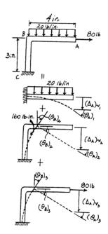
**12–101.** The W24  $\times$  104 A-36 steel beam is used to support the uniform distributed load and a concentrated force which is applied at its end. If the force acts at an angle with the vertical as shown, determine the horizontal and vertical displacement at point A.
