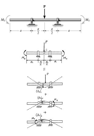
**12–94.** The beam supports the loading shown. Code restrictions, due to a plaster ceiling, require the maximum deflection not to exceed 1/360 of the span length. Select the lightest-weight A-36 steel wide-flange beam from Appendix B that will satisfy this requirement and safely support the load. The allowable bending stress is  $\sigma_{\rm allow}=24$  ksi and the allowable shear stress is  $\tau_{\rm allow}=14$  ksi. Assume A is a roller and B is a pin.
