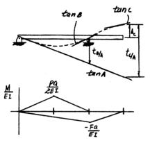
$$t_{B/A} = \frac{1}{2} \left( \frac{Pa}{2EI} \right) (2a)(a) + \frac{1}{2} \left( -\frac{Fa}{EI} \right) (2a) \left( \frac{2}{3} a \right) = \frac{Pa^3}{2EI} - \frac{2Fa^3}{3EI}$$
