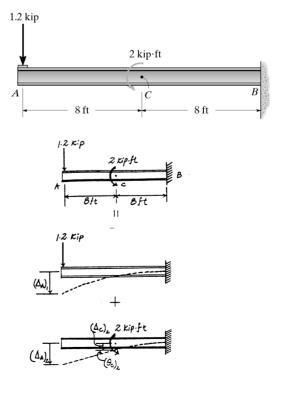
**12–90.** The W8  $\times$  48 cantilevered beam is made of A-36 steel and is subjected to the loading shown. Determine the deflection at C and the slope at A.
