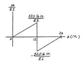
12-61. The beam is subjected to the loading shown. Determine the slope at A and the displacement at C. Assume the support at A is a pin and B is a roller. EI is constant.
