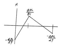
**12–105.** Determine the reactions at the supports A, B, and C; then draw the shear and moment diagrams. EI is constant.
