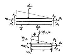
**12–143.** Using the method of superposition, determine the magnitude of  $\mathbf{M}_0$  in terms of the distributed load w and dimension a so that the deflection at the center of the beam is zero. EI is constant.
