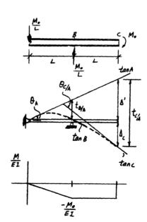
\*12-64. If the bearings at A and B exert only vertical reactions on the shaft, determine the slope at A. EI is constant.
