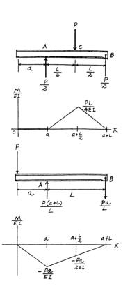
**12–70.** The beam is made of a ceramic material. In order to obtain its modulus of elasticity, it is subjected to the elastic loading shown. If the moment of inertia is I and the beam has a measured maximum deflection  $\Delta$ , determine E.
