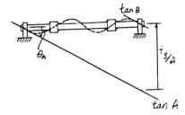
**12–65.** If the bearings at A and B exert only vertical reactions on the shaft, determine the slope at C. EI is constant.
