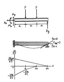
**\*12–116.** Determine the reactions at the supports, then draw the shear and moment diagrams. *EI* is constant.
