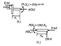
12–18. Determine the equations of the elastic curve using the coordinates  $x_1$  and  $x_2$ , and specify the deflection and slope at C. EI is constant.
