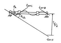
**12–66.** Determine the deflection at C and the slope of the beam at A, B, and C. EI is constant.
