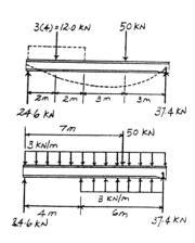
\*12-40. The beam is subjected to the loads shown. Determine the equation of the elastic curve. EI is constant.
