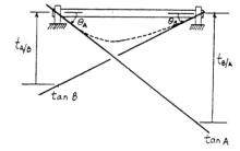
**12–75.** Determine the maximum deflection of the 50-mm-diameter A-36 steel shaft. It is supported by bearings at its ends A and B which only exert vertical reactions on the shaft.
