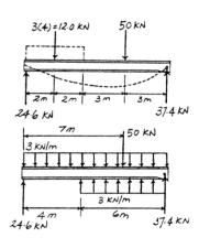
12-39. The beam is subjected to the load shown. Determine the displacement at x = 7 m and the slope at A. EI is constant.
