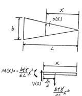
12-30. The beam is made of a material having a specific weight  $\gamma$ . Determine the displacement and slope at its end A due to its weight.
