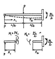
**12–13.** The fence board weaves between the three smooth fixed posts. If the posts remain along the same line, determine the maximum bending stress in the board. The board has a width of 6 in. and a thickness of 0.5 in.  $E = 1.60(10^3)$  ksi. Assume the displacement of each end of the board relative to its center is 3 in.
