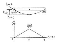
\*12–60. The shaft is supported by a journal bearing at A, which exerts only vertical reactions on the shaft, and by a thrust bearing at B, which exerts both horizontal and vertical reactions on the shaft. Determine the slope of the shaft at the bearings. EI is constant.
