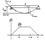
**12–71.** Determine the maximum deflection of the shaft. EI is constant. The bearings exert only vertical reactions on the shaft.
