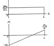
\*12–104. Determine the reactions at the supports A and B, then draw the shear and moment diagrams. EI is constant. Neglect the effect of axial load.
