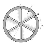
**Centrifugal Force:** The centrifugal force acting on a unit length of the rim rotating at a constant rate of  $\omega$  is
