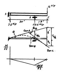
**12–55.** Determine the slope and deflection at *B. EI* is constant.
