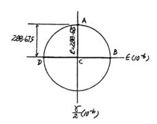
\*10-52. A material is subjected to principal stresses  $\sigma_x$  and  $\sigma_y$ . Determine the orientation  $\theta$  of a strain gauge placed at the point so that its reading of normal strain responds only to  $\sigma_y$  and not  $\sigma_x$ . The material constants are E and  $\nu$ .
