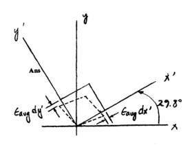
**10–9.** The state of strain at the point on the spanner wrench has components of  $\epsilon_x = 260(10^{-6})$ ,  $\epsilon_y = 320(10^{-6})$ , and  $\gamma_{xy} = 180(10^{-6})$ . Use the strain-transformation equations to determine (a) the in-plane principal strains and (b) the maximum in-plane shear strain and average normal strain. In each case specify the orientation of the element and show how the strains deform the element within the x-y plane.
