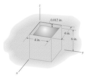
Normal Strains: Since the aluminum is confined at its sides by a rigid container and allowed to expand in the z direction,  $\varepsilon_x = \varepsilon_y = 0$ ; whereas  $\varepsilon_z = \frac{0.012}{6} = 0.002$ . Applying the generalized Hooke's Law with the additional thermal strain,
