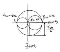
Construction of the Circle  $(x-y \ Plane)$ : In accordance with the sign convention,  $\varepsilon_x = -480 \left(10^{-6}\right)$ ,  $\varepsilon_y = 650 \left(10^{-6}\right)$ , and  $\frac{\gamma_{xy}}{2} = 390 \left(10^{-6}\right)$ . Hence,
