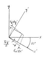
**10–5.** Due to the load **P**, the state of strain at the point on the bracket has components of  $\epsilon_x = 500(10^{-6})$ ,  $\epsilon_y = 350(10^{-6})$ , and  $\gamma_{xy} = -430(10^{-6})$ . Use the straintransformation equations to determine the equivalent inplane strains on an element oriented at an angle of  $\theta = 30^{\circ}$  clockwise from the original position. Sketch the deformed element due to these strains with in the x-y plane.
