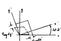
**10–11.** The state of strain at the point on the fan blade has components of  $\epsilon_x = 250(10^{-6})$ ,  $\epsilon_y = -450(10^{-6})$ , and  $\gamma_{xy} = -825(10^{-6})$ . Use the strain-transformation equations to determine (a) the in-plane principal strains and (b) the maximum in-plane shear strain and average normal strain. In each case specify the orientation of the element and show how the strains deform the element within the *x*-*v* plane.
