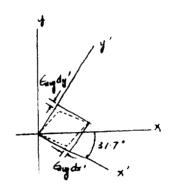
10-7. The state of strain at the point on the gear tooth has components of  $\epsilon_x = 850(10^{-6})$ ,  $\epsilon_y = 480(10^{-6})$ ,  $\gamma_{xy} = 650(10^{-6})$ . Use the strain-transformation equations to determine (a) the in-plane principal strains and (b) the maximum in-plane shear strain and average normal strain. In each case specify the orientation of the element and show how the strains deform the element within the x-y plane.
