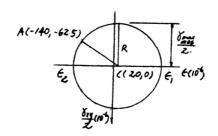
**10–27.** The steel bar is subjected to the tensile load of 500 lb. If it is 0.5 in. thick determine the absolute maximum shear strain.  $E = 29(10^3)$  ksi,  $\nu = 0.3$ .
