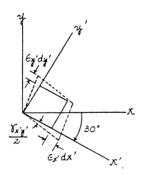
10-6. The state of strain at the point on a wrench has components  $\epsilon_x = 120(10^{-6})$ ,  $\epsilon_y = -180(10^{-6})$ ,  $\gamma_{xy} = 120(10^{-6})$  $150(10^{-6})$ . Use the strain-transformation equations to determine (a) the in-plane principal strains and (b) the maximum inplane shear strain and average normal strain. In each case specify the orientation of the element and show how the strains deform the element within the x-y plane.
