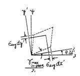
**10–23.** The strain at point A on the bracket has components  $\epsilon_x = 300(10^{-6})$ ,  $\epsilon_y = 550(10^{-6})$ ,  $\gamma_{xy} = -650(10^{-6})$ ,  $\epsilon_z = 0$ . Determine (a) the principal strains at A, (b) the maximum shear strain in the x-y plane, and (c) the absolute maximum shear strain.
