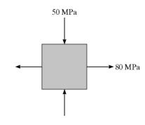
**10–82.** The state of stress acting at a critical point on a machine element is shown in the figure. Determine the smallest yield stress for a steel that might be selected for the part, based on the maximum-shear-stress theory.
