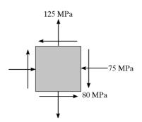
**10–66.** The components of plane stress at a critical point on an A-36 structural steel shell are shown. Determine if failure (yielding) has occurred on the basis of the maximum-distortion-energy theory.
