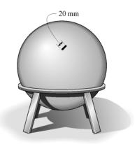
Normal Stresses: Since  $\frac{r}{t} = \frac{1000}{10} = 100 > 10$ , the thin wall analysis is valid to determine the normal stress in the wall of the spherical vessel. This is a plane stress problem where  $\sigma_{\min} = 0$  since there is no load acting on the outer surface of the wall.
