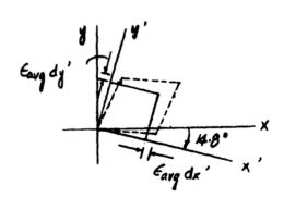
\*10-8. The state of strain at the point on the gear tooth has the components  $\epsilon_x = 520(10^{-6}), \ \epsilon_y = -760(10^{-6}),$  $\gamma_{xv} = -750(10^{-6})$ . Use the strain-transformation equations to determine (a) the in-plane principal strains and (b) the maximum in-plane shear strain and average normal strain. In each case specify the orientation of the element and show how the strains deform the element within the x-y plane.
