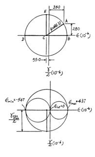
Construction of the Circle (x-y Plane): In accordance with the sign convention,  $\varepsilon_x = 350 \left(10^{-6}\right)$ ,  $\varepsilon_y = -460 \left(10^{-6}\right)$ , and  $\frac{\gamma_{xy}}{2} = -280 \left(10^{-6}\right)$ . Hence,
