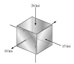
Normal Strains: Applying the generalized Hooke's Law with  $\sigma_z = 10$  ksi,  $\sigma_v = -15$  ksi, and  $\sigma_z = -26$  ksi.
