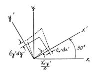
**10–3.** The state of strain at the point on the pin leaf has components of  $\epsilon_x = 200(10^{-6})$ ,  $\epsilon_y = 180(10^{-6})$ , and  $\gamma_{xy} = -300(10^{-6})$ . Use the strain-transformation equations and determine the equivalent in-plane strains on an element oriented at an angle of  $\theta = 60^{\circ}$  counterclockwise from the original position. Sketch the deformed element due to these strains within the x-y plane.
