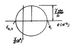
\*10–28. The 45° strain rosette is mounted on the surface of an aluminum plate. The following readings are obtained for each gauge:  $\epsilon_a = 475(10^{-6})$ ,  $\epsilon_b = 250(10^{-6})$ , and  $\epsilon_c = -360(10^{-6})$ . Determine the in-plane principal strains.
