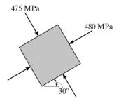
10-81. The principal plane stresses acting on a differential element are shown. If the material is machine steel having a yield stress of  $\sigma_Y = 700 \text{ MPa}$ , determine the factor of safety with respect to yielding if the maximum-shear-stress theory is considered.
