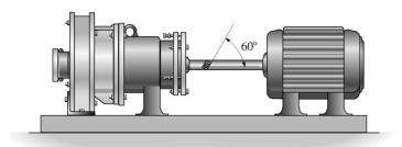
$$\omega = (1760 \text{ rev/min})(\frac{1 \text{ min}}{60 \text{ sec}})(\frac{2\pi \text{ rad}}{1 \text{ rev}}) = 184.307 \text{ rad/s}$$
