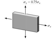
**10–74.** The plate is made of Tobin bronze, which yields at  $\sigma_Y = 25$  ksi. Using the maximum-distortion-energy theory, determine the maximum tensile stress  $\sigma_x$  that can be applied to the plate if a tensile stress  $\sigma_y = 0.75\sigma_x$  is also applied.
