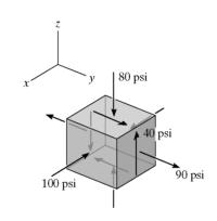
Construction of the Circle: Mohr's circle for the element in the y-z plane is drawn first. In accordance with the sign convention,  $\sigma_y=90$  psi,  $\sigma_z=-80$  psi, and  $\tau_{yz}=40$  psi. Hence,
