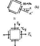
**9–18.** The steel bar has a thickness of 0.5 in. and is subjected to the edge loading shown. Determine the principal stresses developed in the bar.
