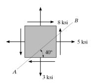
\*9-8. Solve Prob. 9-4 using the stress-transformation equations developed in Sec. 9.2.
