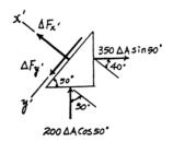
\*9-4. The state of stress at a point in a member is shown on the element. Determine the stress components acting on the inclined plane AB. Solve the problem using the method of equilibrium described in Sec. 9.1.
