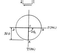
\*9–76. Determine (a) the principal stress and (b) the maximum in-plane shear stress and average normal stress. Specify the orientation of the element in each case.
