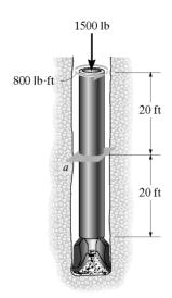
Internal Forces and Torque: As shown on FBD (a).
