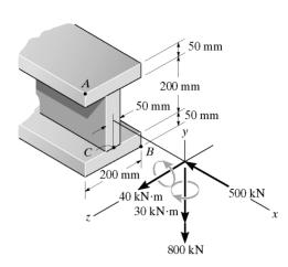
9-39. The wide-flange beam is subjected to the 50-kN force. Determine the principal stresses in the beam at point A located on the web at the bottom of the upper flange. Although it is not very accurate, use the shear formula to calculate the shear stress.
