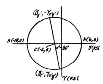
9-101. The internal loadings on a cross section through the 6-in.-diameter drive shaft of a turbine consist of an axial force of 2500 lb, a bending moment of 800 lb · ft. and a torsional moment of 1500 lb · ft. Determine the principal stresses at point A. Also compute the maximum in-plane shear stress at this point.
