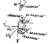
**9–6.** The state of stress at a point in a member is shown on the element. Determine the stress components acting on the inclined plane AB. Solve the problem using the method of equilibrium described in Sec. 9.1.
