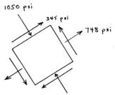
**9–11.** Determine the equivalent state of stress on an element if the element is oriented  $60^{\circ}$  clockwise from the element shown.
