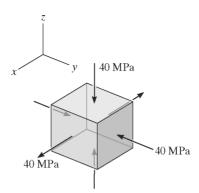
Three Mohr's Circles:  $\sigma_{\text{max}} = 40 \text{ MPa}$   $\sigma_{\text{int}} = \sigma_{\text{min}} = -40 \text{ MPa}$
