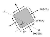
**9–10.** Determine the equivalent state of stress on an element if the element is oriented 30° counterclockwise from the element shown. Use the stress-transformation equations.
