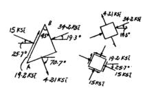
\*9-16. The state of stress at a point is shown on the element. Determine (a) the principal stresses and (b) the maximum in-plane shear stress and average normal stress at the point. Specify the orientation of the element in each case.
