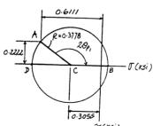
**9–83.** The stair tread of the escalator is supported on two of its sides by the moving pin at A and the roller at B. If a man having a weight of 300 lb stands in the center of the tread, determine the principal stresses developed in the supporting truck on the cross section at point C. The stairs move at constant velocity.
