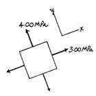
\*9-20. The stress acting on two planes at a point is indicated. Determine the shear stress on plane a-a and the principal stresses at the point.
