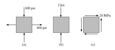
a) Construction of the Circle: In accordance with the sign convention,  $\sigma_x = 800$  psi,  $\sigma_y = -600$  psi, and  $\tau_{xy} = 0$ . Hence,
