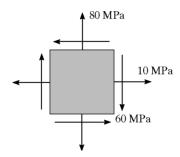
Construction of the Circle: In accordance with the sign convention,  $\sigma_x = 10$  MPa,  $\sigma_y = 80$  MPa and  $\tau_{xy} = -60$  MPa. Hence.
