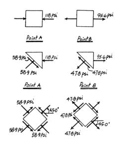
Orientation of the plane for Maximum In-Plane Shear Stress: Applying Eq. 9-6 for point A.
