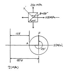
\*9-100. Determine the equivalent state of stress if an element is oriented 40° clockwise from the element shown. Use Mohr's circle.
