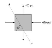
**9–9.** Solve Prob. 9–6 using the stress-transformation equations developed in Sec. 9.2. Show the result on a sketch.
