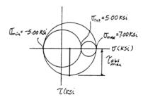
**\*9–92.** The stress at a point is shown on the element. Determine the principal stresses and the absolute maximum shear stress.
