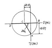
\*9-84. The pedal crank for a bicycle has the cross section shown. If it is fixed to the gear at B and does not rotate while subjected to a force of 75 lb, determine the principal stresses in the material on the cross section at point C.
