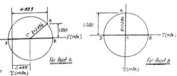
In Plane Principal Stresses: The coordinates of points B and D represent  $\sigma_1$  and  $\sigma_2$ , respectively. For point A
