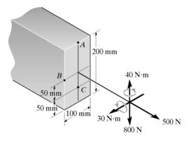
9-53. The internal loadings at a section of the beam consist of an axial force of 500 N, a shear force of 800 N, and two moment components of 30 N·m and 40 N·m. Determine the principal stresses at point C. Also calculate the maximum in-plane shear stress at this point.
