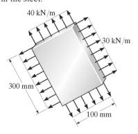
Normal and Shear Stress: In accordance with the established sign convention,
