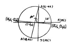
\*9–80. Mohr's circle for the state of stress in Fig. 9–15a is shown in Fig. 9-15b. Show that finding the coordinates of point  $P(\sigma_{x'}, \tau_{x'y'})$  on the circle gives the same value as the stress-transformation Eqs. 9-1 and 9-2.
