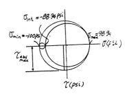
**9–91.** The stress at a point is shown on the element. Determine the principal stresses and the absolute maximum shear stress.
