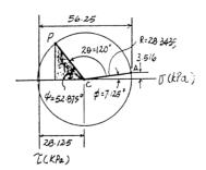
**9–86.** The frame supports the distributed loading of 200 N/m. Determine the normal and shear stresses at point E that act perpendicular and parallel, respectively, to the grains. The grains at this point make an angle of  $60^{\circ}$  with the horizontal as shown.
