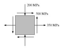
Construction of the Circle: In accordance with the sign convention,  $\sigma_x = 350$  MPa,  $\sigma_y = -200$  MPa, and  $\tau_{xy} = 500$  MPa. Hence,
