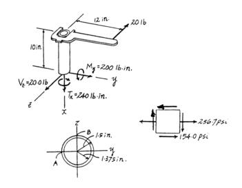
\*9-48. The cantilevered beam is subjected to the load at its end. Determine the principal stresses in the beam at points A and B.
