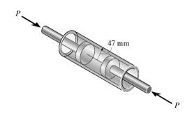
\*8-68. Determine the maximum force P that can be exerted on each of the two pistons so that the circumferential stress component in the cylinder does not exceed 3 MPa. Each piston has a radius of 45 mm and the cylinder has a wall thickness of 2 mm.
