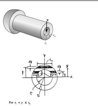
$$\tau = \frac{\frac{2}{3}V\left[\left(r_{o}^{2} - y^{2}\right)^{\frac{1}{2}}\right]}{\frac{\pi}{4}\left(\left(r_{o}^{4} - r_{i}^{4}\right)(2)\left(r_{o}^{2} - y^{2}\right)^{\frac{1}{2}}\right]}$$
