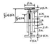
**7-42.** The beam is fabricated from two equivalent structural tees and two plates. Each plate has a height of 6 in. and a thickness of 0.5 in. If the bolts are spaced at s = 8 in., determine the maximum shear force V that can be applied to the cross section. Each bolt can resist a shear force of 15 kip.
