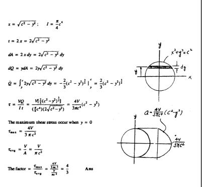
**\*7–20.** Develop an expression for the average vertical component of shear stress acting on the horizontal plane through the shaft, located a distance y from the neutral axis.
