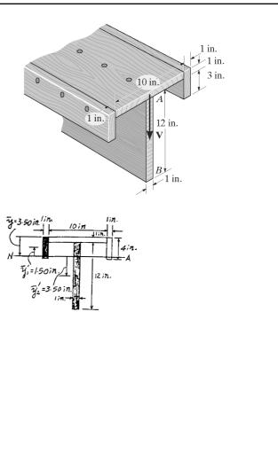
**7–85.** The beam is constructed from four boards glued together at their seams. If the glue can withstand 75 lb/in., what is the maximum vertical shear V that the beam can support?
