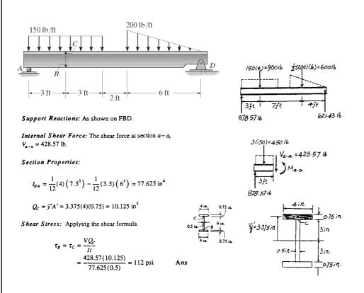
**\*7–28.** Determine the maximum shear stress acting in the fiberglass beam at the critical section.
