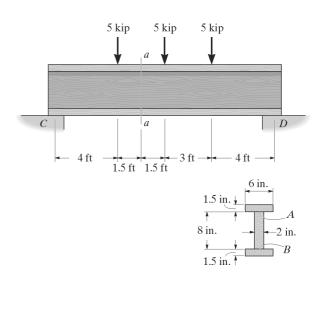
**7–27.** Determine the shear stress at points B and C located on the web of the fiberglass beam.
