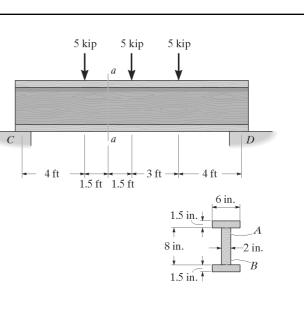
**7–25.** The beam is made from three boards glued together at the seams A and B. If it is subjected to the loading shown, determine the maximum shear stress developed in the glued joints. The supports at C and D exert only vertical reactions on the beam.
