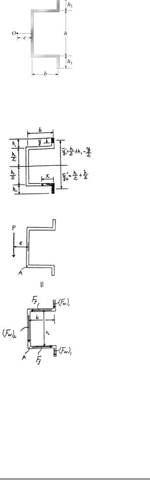
**7-74.** Determine the location e of the shear center, point O, for the thin-walled member having the cross section shown. The member segments have the same thickness t.
