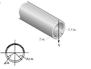
\*7-12. The strut is subjected to a vertical shear of V = 130 kN. Plot the intensity of the shear-stress distribution acting over the cross-sectional area, and compute the resultant shear force developed in the vertical segment *AB*.
