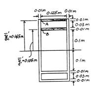
**7–57.** A shear force of V = 18 kN is applied to the box girder. Determine the shear flow at C.
