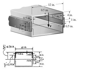
**7–50.** The strut is constructed from three pieces of plastic that are glued together as shown. If the allowable shear stress for the plastic is  $\tau_{\text{allow}} = 800$  psi and each glue joint can withstand 250 lb/in., determine the largest allowable distributed loading w that can be applied to the strut.
