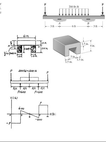
**7–18.** If the force P = 800 lb, determine the maximum shear stress in the beam at the critical section. The supports at A and B only exert vertical reactions on the beam.
