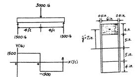
\*7-44. The double-web girder is constructed from two plywood sheets that are secured to wood members at its top and bottom. The allowable bending stress for the wood is  $\sigma_{\text{allow}} = 8 \text{ ksi}$  and the allowable shear stress is  $\tau_{\text{allow}} = 3 \text{ ksi}$ . If the fasteners are spaced s = 6 in. and each fastener can support 600 lb in single shear, determine the maximum load P that can be applied to the beam.
