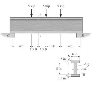
**7–26.** The beam is made from three boards glued together at the seams A and B. If it is subjected to the loading shown, determine the maximum vertical shear force resisted by the top flange of the beam. The supports at C and D exert only vertical reactions on the beam.
