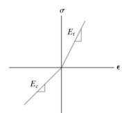
**6–101.** The beam has a rectangular cross section and is subjected to a bending moment M. If the material from which it is made has a different modulus of elasticity for tension and compression as shown, determine the location c of the neutral axis and the maximum compressive stress in the beam.
