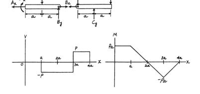
\*6–12. Draw the shear and moment diagrams for the compound beam which is pin connected at *B*.
