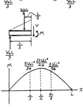
**6–30.** Draw the shear and moment diagrams for the beam.
