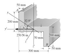
\*6-116. Using the techniques outlined in Appendix A, Example A.5 or A.6, the Z section has principal moments of inertia of  $I_y = 0.060(10^{-3}) \,\mathrm{m}^4$  and  $I_z = 0.471(10^{-3}) \,\mathrm{m}^4$ , computed about the principal axes of inertia y and z, respectively. If the section is subjected to an internal moment of  $M = 250 \,\mathrm{N} \cdot \mathrm{m}$  directed horizontally as shown, determine the stress produced at point B. Solve the problem using Eq. 6-17.
