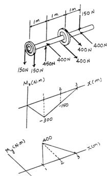
**6–109.** The shaft is subjected to the vertical and horizontal loadings of two pulleys D and E as shown. It is supported on two journal bearings at A and B which offer no resistance to axial loading. Furthermore, the coupling to the motor at C can be assumed not to offer any support to the shaft. Determine the required diameter d of the shaft if the allowable bending stress for the material is  $\sigma_{\rm allow} = 180$  MPa.
