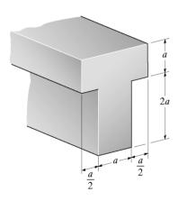
Maximum Elastic Moment: The centroid and the moment of inertia about neutral axis must be determined first.
