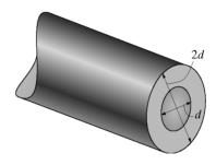
Maximum Elastic Moment: The moment of inertia about neutral axis must be determined first.
