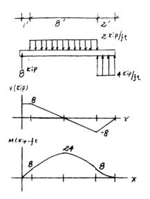
**6–25.** Draw the shear and moment diagrams for the beam. The two segments are joined together at B.
