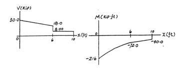
Absolute Maximum Bending Stress: The maximum moment is  $M_{\rm max}=216~{\rm kip}\cdot{\rm ft}$  as indicated on moment diagram. Applying the flexure formula
