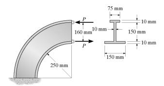
Internal Moment:  $M = 0.160(6) = 0.960 \text{ kN} \cdot \text{m}$  is positive since it tends to increase the beam's radius of curvature.
