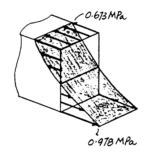
**6–141.** The member has an elliptical cross section. If it is subjected to a moment of  $M = 50 \,\mathrm{N} \cdot \mathrm{m}$ , determine the stress at points A and B. Is the stress at point A', which is located on the member near the wall, the same as that at A? Explain.
