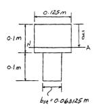
**6–126.** The composite beam is made of A-36 steel (A) bonded to C83400 red brass (B) and has the cross section shown. If the allowable bending stress for the steel is  $(\sigma_{\rm allow})_{\rm st} = 180$  MPa and for the brass  $(\sigma_{\rm allow})_{\rm br} = 60$  MPa, determine the maximum moment M that can be applied to the beam.
