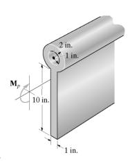
\*6–168. Determine the plastic section modulus and the shape factor for the member having the tubular cross section.
