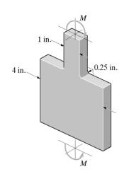
**6–145.** The bar is subjected to a moment of  $M = 40 \text{ N} \cdot \text{m}$ . Determine the smallest radius r of the fillets so that an allowable bending stress of  $\sigma_{\rm allow} = 124 \, \mathrm{MPa}$  is not exceeded.
