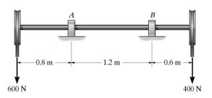
**6–73.** Determine the smallest allowable diameter of the shaft which is subjected to the concentrated forces. The sleeve bearings at A and B support only vertical forces, and the allowable bending stress is  $\sigma_{\rm allow} = 160$  MPa.
