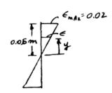
**6–178.** The bar is made of an aluminum alloy having a stress–strain diagram that can be approximated by the straight line segments shown. Assuming that this diagram is the same for both tension and compression, determine the moment the bar will support if the maximum strain at the top and bottom fibers of the beam is  $\epsilon_{\rm max} = 0.03$ .
