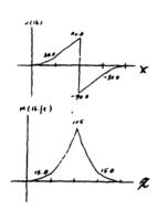
**6–33.** Draw the shear and moment diagrams for the beam.
