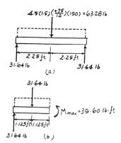
\*6–48. The slab of marble, which can be assumed a linear elastic brittle material, has a specific weight of 150 lb/ft<sup>3</sup>. If it is supported on its edges as shown in (b), determine the minimum thickness it should have without causing it to break. The fracture stress is  $\sigma_f = 200$  psi.
