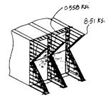
**6–123.** The steel channel is used to reinforce the wood beam. Determine the maximum stress in the steel and in the wood if the beam is subjected to a moment of  $M=850\,\mathrm{lb}\cdot\mathrm{ft}$ .  $E_{\mathrm{st}}=29(10^3)\,\mathrm{ksi}$ ,  $E_{\mathrm{w}}=1600\,\mathrm{ksi}$ .
