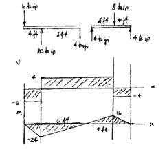
**6–13.** Draw the shear and moment diagrams for the beam.
