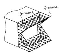
**6–47.** The slab of marble, which can be assumed a linear elastic brittle material, has a specific weight of  $150 \text{ lb/ft}^3$  and a thickness of 0.75 in. Calculate the maximum bending stress in the slab if it is supported (a) on its side and (b) on its edges. If the fracture stress is  $\sigma_f = 200 \text{ psi}$ , explain the consequences of supporting the slab in each position.
