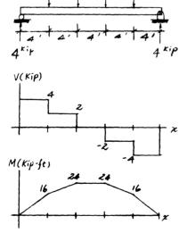
**6–5.** A reinforced concrete pier is used to support the stringers for a bridge deck. Draw the shear and moment diagrams for the pier when it is subjected to the stringer loads shown. Assume the columns at A and B exert only vertical reactions on the pier.
