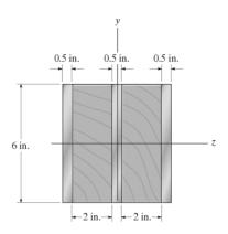
Section Properties: For the transformed section.
