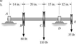
\*6-4. Draw the shear and moment diagrams for the beam.
