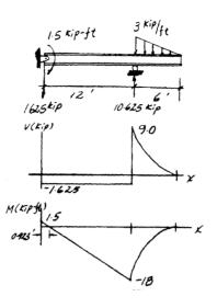
**6–37.** The compound beam consists of two segments that are pinned together at B. Draw the shear and moment diagrams if it supports the distributed loading shown.
