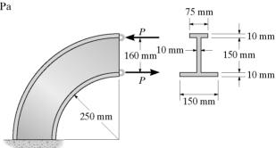
Allowable Normal Stress: Applying the curved - beam formula
