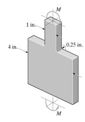
\*6-144. The bar has a thickness of 0.5 in. and is subjected to a moment of 60 lb · ft. Determine the maximum bending stress in the bar.
