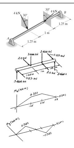
**6–113.** The steel shaft is subjected to the two loads that act in the directions shown. If the journal bearings at A and B do not exert an axial force on the shaft, determine the required diameter of the shaft if the allowable bending stress is  $\sigma_{\rm allow} = 180 \, {\rm MPa}$ .
