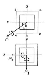
\*6–104. The beam has a rectangular cross section. If it is subjected to a bending moment of  $M = 3500 \,\mathrm{N} \cdot \mathrm{m}$  directed as shown, determine the maximum bending stress in the beam and the orientation of the neutral axis.
