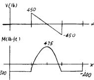
**6–22.** Draw the shear and moment diagrams for the compound beam. The three segments are connected by pins at B and E.
