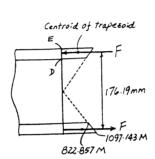
**6–46.** Determine the moment M that should be applied to the beam in order to create a compressive stress at point D of  $\sigma_D = 30$  MPa. Also sketch the stress distribution acting over the cross section and compute the maximum stress developed in the beam.
