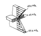
\*6-56. The beam is made from three boards nailed together as shown. If the moment acting on the cross section is  $M = 1 \text{ kip} \cdot \text{ft}$ , determine the maximum bending stress in the beam. Sketch a three-dimensional view of the stress distribution acting over the cross section.
