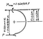
Allowable Normal Stress: Applying the curved - beam formula
