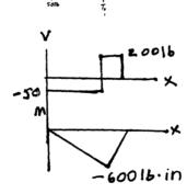
**6–3.** Draw the shear and moment diagrams for the shaft. The bearings at A and D exert only vertical reactions on the shaft. The loading is applied to the pulleys at B and C and E.
