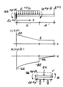
**6–185.** Draw the shear and moment diagrams for the beam. *Hint:* The 20-kip load must be replaced by equivalent loadings at point *C* on the axis of the beam.
