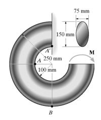
6-142. The member has an elliptical cross section. If the allowable bending stress is  $\sigma_{\text{allow}} = 125 \text{ MPa}$ , determine the maximum moment M that can be applied to the
