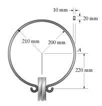
Maximum Normal Stress: Applying the curved - beam formula
