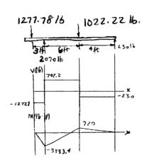
\*6–96. The beam supports the load of 5 kip. Determine the absolute maximum bending stress in the beam if the sides of its triangular cross section are a = 6 in.
