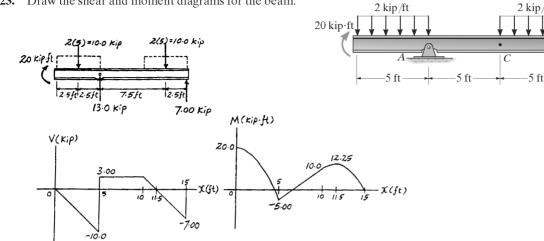
\*6-24. The beam is bolted or pinned at A and rests on a bearing pad at B that exerts a uniform distributed loading on the beam over its 2-ft length. Draw the shear and moment diagrams for the beam if it supports a uniform loading of 2 kip/ft.
