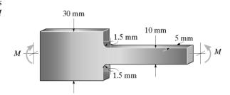
**6–149.** Determine the maximum bending stress developed in the bar if it is subjected to the couples shown. The bar has a thickness of 0.25 in.
