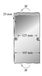
\*6–152. The stepped bar has a thickness of 15 mm. Determine the maximum moment that can be applied to its ends if it is made of a material having an allowable bending stress of  $\sigma_{\rm allow} = 200 \, {\rm MPa}$ .
