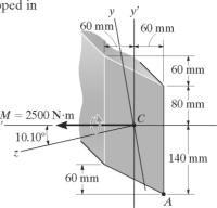
$$\sigma_{A} = \frac{-(M_{z} \cdot I_{y'} + M_{y'} \cdot I_{y'z'})y' + (M_{y'} \cdot I_{z'} + M_{z'} \cdot I_{y'z'})z'}{I_{y'} I_{z'} - I_{y'z'}^{2}}$$
