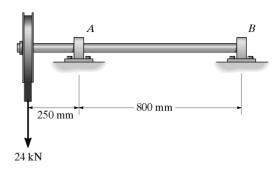
**6–62.** If the shaft in Prob. 6–3 has a diameter of 1.5 in., determine the absolute maximum bending stress in the shaft.
