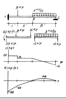
**6–27.** Determine the placement distance a of the roller support so that the largest absolute value of the moment is a minimum. Draw the shear and moment diagrams for this condition.
