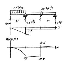
\*6–20. Draw the shear and moment diagrams for the beam, and determine the shear and moment throughout the beam as functions of x.
