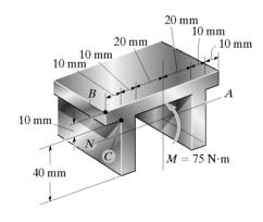
6-53. A beam is constructed from four pieces of wood, glued together as shown. If the moment acting on the cross section is  $M = 450 \,\mathrm{N} \cdot \mathrm{m}$ , determine the resultant force the bending stress produces on the top board A and on the side
