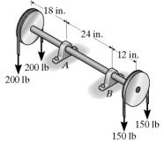
Absolute Maximum Bending Stress: The maximum moment is  $M_{\rm max} = 7200 \ {\rm lb} \cdot {\rm in}$  as indicated on moment diagram. Applying the flexure formula
