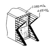
**6–125.** The composite beam is made of A-36 steel (A) bonded to C83400 red brass (B) and has the cross section shown. If it is subjected to a moment of  $M = 6.5 \text{ kN} \cdot \text{m}$ , determine the maximum stress in the brass and steel. Also, what is the stress in each material at the seam where they are bonded together?
