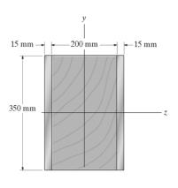
Section Properties: For the transformed section.
