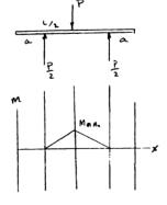
**6–82.** If the beam in Prob. 6–23 has a cross section as shown, determine the absolute maximum bending stress in the beam.
