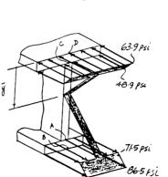
**6-57.** Determine the resultant force the bending stresses produce on the top board A of the beam if  $M = 1 \text{ kip} \cdot \text{ft}$ .
