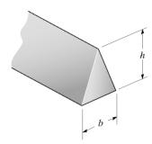
Maximum Elastic Moment: Applying the flexure formula with  $\sigma = \sigma_y$ , we have
