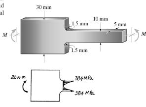
\*6-148. The allowable bending stress for the bar is  $\sigma_{\text{allow}} = 175 \text{ MPa}$ . Determine the maximum moment M that can be applied to the bar.
