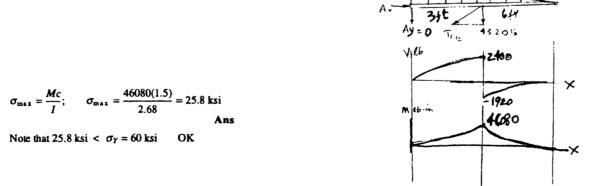
**6–95.** The boat has a weight of 2300 lb and a center of gravity at G. If it rests on the trailer at the smooth contact A and can be considered pinned at B, determine the absolute maximum bending stress developed in the main strut of the trailer. Consider the strut to be a box-beam having the dimensions shown and pinned at C.
