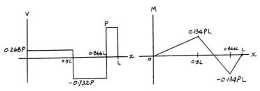
**6–41.** Draw the shear and moment diagrams for the beam.
