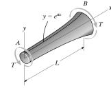
$$\phi = \int \frac{T \, dx}{J(x)G} \quad \text{where, } J(x) = \frac{\pi}{2} (e^{ax})^4$$
