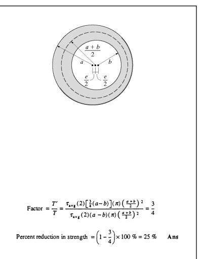
**5–109.** For a given average shear stress, determine the factor by which the torque-carrying capacity is increased if the half-circular sections are reversed from the dashed-line positions to the section shown. The tube is 0.1 in. thick.
