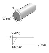
Elastic - Plastic Torque : The maximum elastic torque is  $T_Y = \frac{\pi}{2} \tau_Y c^3 = \frac{\pi}{2} (150) (10^6) (0.02^3) = 1.885 \text{ kN} \cdot \text{m}$  and the plastic torque is  $T_P = \frac{2\pi}{3} \tau_Y c^3 = \frac{2\pi}{3} (150) (10^6) (0.02^3)$   $= 2.513 \text{ kN} \cdot \text{m}$ . Since  $T_Y < T < T_P$ , applying Eq. 5 - 26 from the text, we have
