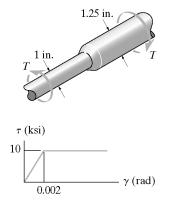
Plastic Torque : For the smaller - diameter segment
