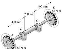
$\phi_{AD} = \Sigma \frac{TL}{JG}$   $= \frac{2(85)(0.4)}{\frac{\pi}{2}(0.015^4 - 0.01^4)(75)(10^9)} + \frac{(85)(0.25)}{\frac{\pi}{2}(0.02^4)(75)(10^9)}$   $= 0.01534 \text{ rad} = 0.879^\circ \text{Ans}$
