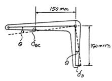
**4–47.** The rigid link is supported by a pin at A, a steel wire BC having an unstretched length of 200 mm and cross-sectional area of 22.5 mm<sup>2</sup>, and a short aluminum block having an unloaded length of 50 mm and cross-sectional area of 40 mm<sup>2</sup>. If the link is subjected to the vertical load shown, determine the rotation of the link about the pin A. Report the answer in radians.  $E_{\rm st} = 200$  GPa,  $E_{\rm al} = 70$  GPa.
