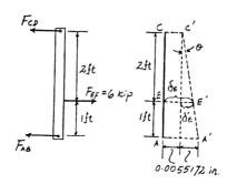
\*4–12. The assembly consists of three titanium (Ti-6A1-4V) rods and a rigid bar AC. The cross-sectional area of each rod is given in the figure. If a force of 6 kip is applied to the ring F, determine the angle of tilt of bar AC.
