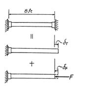
**4-83.** The bronze 86100 pipe has an inner radius of 0.5 in. and a wall thickness of 0.2 in. If the gas flowing through it changes the temperature of the pipe uniformly from  $T_A = 200^{\circ}\mathrm{F}$  at A to  $T_B = 60^{\circ}\mathrm{F}$  at B, determine the axial force it exerts on the walls. The pipe was fitted between the walls when  $T = 60^{\circ}\mathrm{F}$ .
