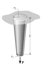
$$\frac{L + x_0}{r_2} = \frac{x_0}{r_1}; \quad x_0 = \frac{L r_1}{r_2 - r_1}$$
