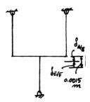
\*4–56. The bar is pinned at A and supported by two aluminum rods, each having a diameter of 1 in. and a modulus of elasticity  $E_{\rm al}=10(10^3)$  ksi. If the bar is assumed to be rigid and initially vertical, determine the displacement of the end B when the force of 2 kip is applied.
