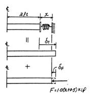
**4-87.** Determine the maximum normal stress developed in the bar when it is subjected to a tension of P = 8 kN.
