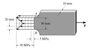
**4–94.** The resulting stress distribution along section AB for the bar is shown. From this distribution, determine the approximate resultant axial force P applied to the bar. Also, what is the stress-concentration factor for this geometry?
