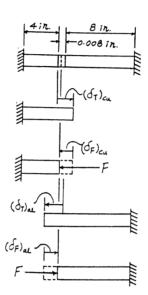
**4-79.** Two bars, each made of a different material, are connected and placed between two walls when the temperature is  $T_1 = 10^{\circ}$ C. Determine the force exerted on the (rigid) supports when the temperature becomes  $T_2 = 20^{\circ}$ C. The material properties and cross-sectional area of each bar are given in the figure.
