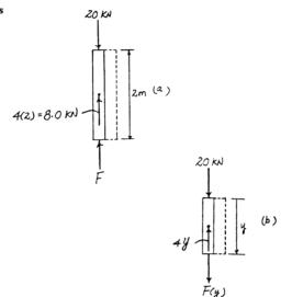
**4–23.** The post is made of Douglas fir and has a diameter of 60 mm. If it is subjected to the load of 20 kN and the soil provides a frictional resistance that is distributed along its length and varies linearly from w = 0 at y = 0 to w = 3 kN/m at y = 2 m, determine the force **F** at its bottom needed for equilibrium. Also, what is the displacement of the top of the post A with respect to its bottom B? Neglect the weight of the post.
