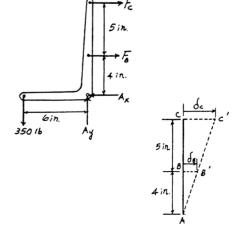
**4–113.** The force **P** is applied to the bar, which is composed of an elastic perfectly plastic material. Construct a graph to show how the force in each section AB and BC (ordinate) varies as P (abscissa) is increased. The bar has cross-sectional areas of 1 in<sup>2</sup> in region AB and 4 in<sup>2</sup> in region BC, and  $\sigma_V = 30$  ksi.
