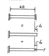
**4–75.** A 6-ft-long steam pipe is made of steel with  $\sigma_Y = 40$  ksi. It is connected directly to two turbines A and B as shown. The pipe has an outer diameter of 4 in. and a wall thickness of 0.25 in. The connection was made at  $T_1 = 70^{\circ}$ F. If the turbines' points of attachment are assumed to have a stiffness of  $k = 80(10^3)$  kip/in., determine the force the pipe exerts on the turbines when the steam and thus the pipe reach a temperature of  $T_2 = 275^{\circ}$ F.
