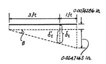
**4–9.** The load is supported by the four 304 stainless steel wires that are connected to the rigid members AB and DC. Determine the angle of tilt of each member after the 500-lb load is applied. The members were originally horizontal, and each wire has a cross-sectional area of 0.025 in<sup>2</sup>.
