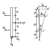
**4–57.** The bar is pinned at A and supported by two aluminum rods, each having a diameter of 1 in. and a modulus of elasticity  $E_{\rm al}=10(10^3)$  ksi. If the bar is assumed to be rigid and initially vertical, determine the force in each rod when the 2-kip load is applied.
