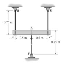
$$\begin{aligned} \mathbf{L} + \mathbf{\Sigma} M_E &= 0; & -T_{AB}(0.5) + T_{CD}(0.5) &= 0 \\ T_{AB} &= T_{CD} &= T \\ + \mathbf{L} \mathbf{\Sigma} F_y &= 0; & T_{EF} - 2T &= 0 \\ T_{EF} &= 2T \end{aligned}$$
