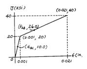
**4–101.** The rigid bar is supported by a pin at A and two steel wires, each having a diameter of 4 mm. If the yield stress for the wires is  $\sigma_Y = 530$  MPa, and  $E_{\rm st} = 200$  GPa, determine the intensity of the distributed load w that can be placed on the beam and will just cause wire EB to yield. What is the displacement of point G for this case? For the calculation, assume that the steel is elastic perfectly plastic.
