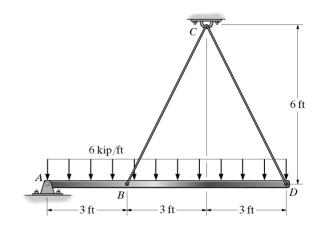
$$\begin{aligned} & \mathbf{f} + \sum M_A = 0; \qquad T_{CB}(\frac{2}{\sqrt{5}})(3) - 54(4.5) + T_{CD}(\frac{2}{\sqrt{5}})9 = 0 \\ & \theta = \tan^{-1}\frac{6}{6} = 45^{\circ} \\ & L_{\theta'C}^2 = (3)^2 + (8.4853)^2 - 2(3)(8.4853)\cos\theta' \end{aligned}$$
