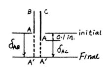
\*4–40. The load of 800 lb is to be supported by the two vertical steel wires for which  $\sigma_Y = 80$  ksi. If, originally, wire AB is 50 in. long and wire AC is 50.1 in. long, determine the cross-sectional area of AB if the load is to be shared equally between both wires. Wire AC has a cross-sectional area of 0.02 in<sup>2</sup>.
