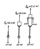
**4–119.** The joint is made from three A-36 steel plates that are bonded together at their seams. Determine the displacement of end A with respect to end B when the joint is subjected to the axial loads shown. Each plate has a thickness of 5 mm.
