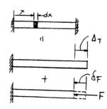
**4-86.** The rod is made of A-36 steel and has a diameter of 0.25 in. If the springs are compressed 0.5 in. when the temperature of the rod is  $T = 40^{\circ}\text{F}$ , determine the force in the rod when its temperature is  $T = 160^{\circ}\text{F}$ .
