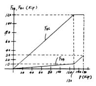
**4–114.** The 2014-T6 aluminum rod has a diameter of 0.5 in. and is lightly attached to the rigid supports at A and B when  $T_1 = 70^{\circ}$ F. If the temperature becomes  $T_2 = -10^{\circ}$ F, and an axial force of P = 16 lb is applied to the rigid collar as shown, determine the reactions at A and B.
