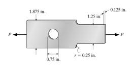
**4–91.** Determine the maximum normal stress developed in the bar when it is subjected to a tension of P = 2 kip.
