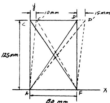
**2-29.** The block is deformed into the position shown by the dashed lines. Determine the shear strain at corners *C* and *D*.
