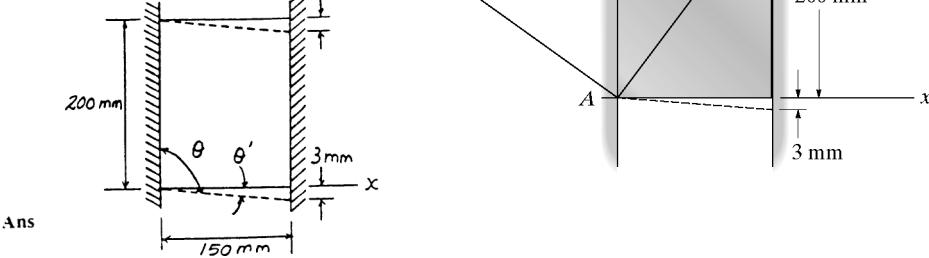
**2-23.** The rectangular plate is subjected to the deformation shown by the dashed lines. Determine the average shear strain  $\gamma_{xy}$  of the plate.
