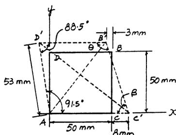
**\*2-20.** The block is deformed into the position shown by the dashed lines. Determine the average normal strain along line AB.
