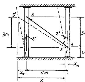
**\*2-16.** The corners of the square plate are given the displacements indicated. Determine the shear strain along the edges of the plate at A and B.
