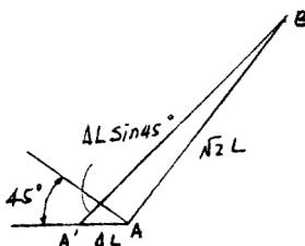
**\*2-12.** The piece of plastic is originally rectangular. Determine the shear strain  $\gamma_{xy}$  at corners A and B if the plastic distorts as shown by the dashed lines.
