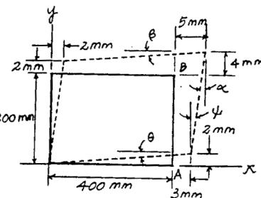
$$(\gamma_A)_{xy} = -(\theta + \psi) \\ = -0.0116 \text{ rad} = -11.6(10^{-3}) \text{ rad}$$
