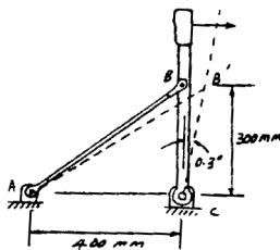
**2–9.** Part of a control linkage for an airplane consists of a rigid member  $CBD$  and a flexible cable  $AB$ . If a force is applied to the end  $D$  of the member and causes a normal strain in the cable of  $0.0035 \text{ mm/mm}$ , determine the displacement of point  $D$ . Originally the cable is unstretched.
