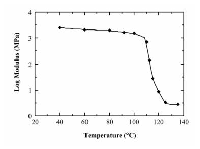
The glass-transition temperature is that temperature corresponding to the abrupt decrease in  $\log E_r(10)$ , which for this PMMA material is about 115°C.
