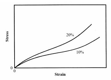
(b) Shown below are the stress-strain curves for the two polypropylene materials. These materials will most probably display the stress-strain behavior of a normal plastic, curve *B* in Figure 15.1. However, the syndiotactic polypropylene has a higher molecular weight and will also undoubtedly have a higher degree of crystallinity; therefore, it will have a higher strength.
