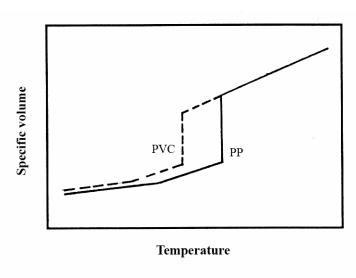
(c) Shown below are specific volume-versus-temperature curves for the polystyrene and polypropylene materials. Since both are totally amorphous, they will exhibit the behavior similar to curve *A* in Figure 15.18. However, since the polystyrene repeat unit has a bulkier side group than polypropylene (Table 14.3), its chain flexibility will be lower, and, thus, its glass-transition temperature will be higher.
