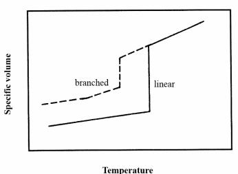
(b) Shown below are specific volume-versus-temperature curves for the poly(vinyl chloride) and polypropylene materials. Since both are 50% crystalline, they will exhibit behavior similar to curve B in Figure 15.18. However, since the polypropylene has the greater molecular weight it will have the higher melting temperature. Furthermore, polypropylene will also have the higher glass-transition temperature inasmuch as its  $CH_3$  side group is bulkier than the Cl for PVC.
