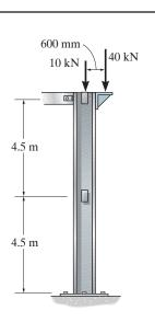
Section Properties. From the table listed in the appendix, the necessary section properties for a W250  $\times$  45 are
