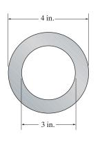
\*13–96. The 2014-T6 aluminum hollow section has the cross section shown. If the column is fixed at its base and pinned at its top, and is subjected to the axial force P = 100 kip, determine the maximum length of the column for it to safely support the load.
