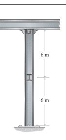
\*13–136. The structural A-36 steel column has the cross section shown. If it is fixed at the bottom and free at the top, determine the maximum force P that can be applied at A without causing it to buckle or yield. Use a factor of safety of 3 with respect to buckling and yielding.
