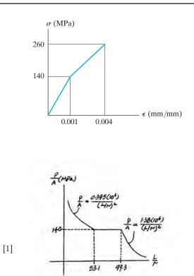
Tangent modulus: From the stress-strain diagram,
