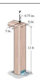
**13–127.** Using the NFPA equations of Sec. 13.6 and Eq. 13–30, determine the maximum allowable eccentric load P that can be applied to the wood column. Assume that the column is pinned at the top and fixed at the bottom.
