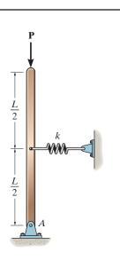
**13–2.** Determine the critical load  $P_{cr}$  for the rigid bar and spring system. Each spring has a stiffness k.
