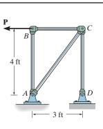
•13–33. The steel bar *AB* of the frame is assumed to be pin connected at its ends for *y*–*y* axis buckling. If w = 3 kN/m, determine the factor of safety with respect to buckling about the *y*–*y* axis due to the applied loading.  $E_{\text{st}} = 200 \text{ GPa}$ ,  $\sigma_Y = 360 \text{ MPa}$ .
