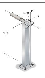
**13–114.** The A-36-steel W10 × 45 column is fixed at its base. Its top is constrained to move along the *x*–*x* axis but free to rotate about and move along the *y*–*y* axis. Determine the maximum eccentric force *P* that can be safely supported by the column using an interaction formula. The allowable bending stress is  $(\sigma_b)_{allow} = 15$  ksi.
