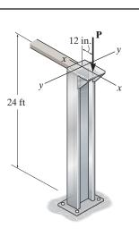
\*13–116. The A-36-steel W12  $\times$  50 column is fixed at its base. Its top is constrained to move along the *x*–*x* axis but free to rotate about and move along the *y*–*y* axis. If the eccentric force P = 15 kip is applied to the column, investigate if the column is adequate to support the loading. Use the interaction formula. The allowable bending stress is  $(\sigma_b)_{allow} = 15$  ksi.
