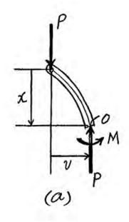
\*13-44. Consider an ideal column as in Fig. 13-10c, having both ends fixed. Show that the critical load on the column is given by  $P_{\rm cr} = 4\pi^2 EI/L^2$ . *Hint*: Due to the vertical deflection of the top of the column, a constant moment  $\mathbf{M}'$  will be developed at the supports. Show that  $d^2v/dx^2 + (P/EI)v = M'/EI$ . The solution is of the form  $v = C_1 \sin(\sqrt{P/EI}x) + C_2 \cos(\sqrt{P/EI}x) + M'/P$ .
