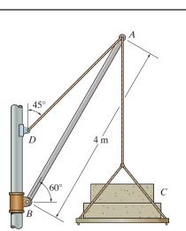
•13–37. If the diameter of the solid L2-steel rod AB is 50 mm, determine the maximum mass C that the rod can support without buckling. Use F.S. = 2 against buckling.
