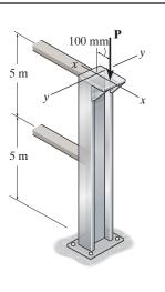
**13–54.** The W200  $\times$  22 A-36-steel column is fixed at its base. Its top is constrained to rotate about the *y*-*y* axis and free to move along the *y*-*y* axis. Also, the column is braced along the *x*-*x* axis at its mid-height. If P = 25 kN, determine the maximum normal stress developed in the column.
