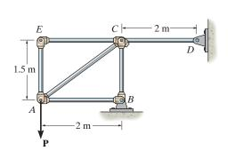
Section the truss through a-a, the FBD of the left cut segment is shown in Fig. a. The compressive force developed in member CB can be obtained directly by writing the force equation of equilibrium along y axis.
