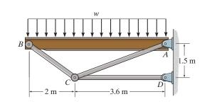
**Equilibrium.** The force developed in member *BC* can be determined by considering the equilibrium of the free-body diagram of the beam *AB*, Fig. *a*.
