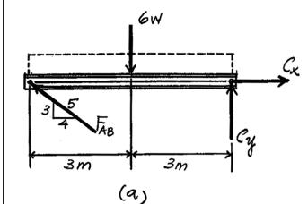
**13–34.** The members of the truss are assumed to be pin connected. If member AB is an A-36 steel rod of 40 mm diameter, determine the maximum force P that can be supported by the truss without causing the member to buckle.
