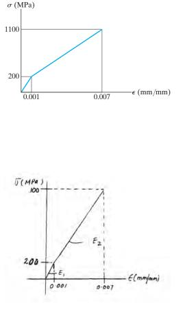
\*13–76. The stress-strain diagram for a material can be approximated by the two line segments shown. If a bar having a diameter of 80 mm and a length of 1.5 m is made from this material, determine the critical load provided the ends are fixed. Assume that the load acts through the axis of the bar. Use Engesser's equation.
