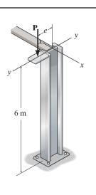
**13–58.** The W250  $\times$  28 A-36-steel column is fixed at its base. Its top is constrained to rotate about the *y*-*y* axis and free to move along the *y*-*y* axis. Determine the force **P** and its eccentricity *e* so that the column will yield and buckle simultaneously.
