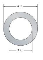
•13–97. The tube is 0.25 in. thick, is made of a 2014-T6 aluminum alloy, and is fixed at its bottom and pinned at its top. Determine the largest axial load that it can support.
