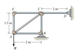
By inspecting the equilibrium of joint E,  $F_{AB} = 0$ . Then, the compressive force developed in member AB can be determined by analysing the equilibrium of joint A, Fig. a.
