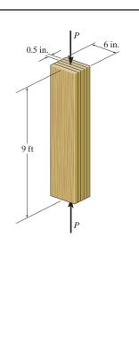
•13–105. The column is made of wood. It is fixed at its bottom and free at its top. Use the NFPA formulas to determine its greatest allowable length if it supports an axial load of P = 2 kip.
