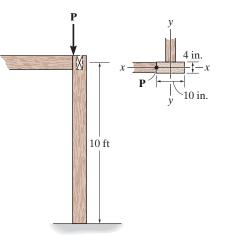
•13–53. The W200 × 22 A-36-steel column is fixed at its base. Its top is constrained to rotate about the y-y axis and free to move along the y-y axis. Also, the column is braced along the x-x axis at its mid-height. Determine the allowable eccentric force P that can be applied without causing the column either to buckle or yield. Use F.S. = 2 against buckling and F.S. = 1.5 against yielding.
