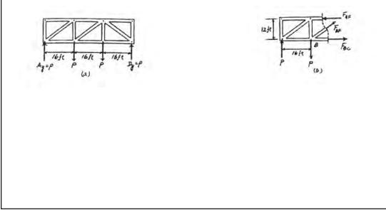
**13–39.** The members of the truss are assumed to be pin connected. If member AG is an A-36 steel rod having a diameter of 2 in., determine the greatest magnitude of load **P** that can be supported by the truss without causing this member to buckle.
