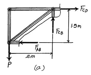
\*13-36. If load *C* has a mass of 500 kg, determine the required minimum diameter of the solid L2-steel rod *AB* to the nearest mm so that it will not buckle. Use F.S. = 2 against buckling.
