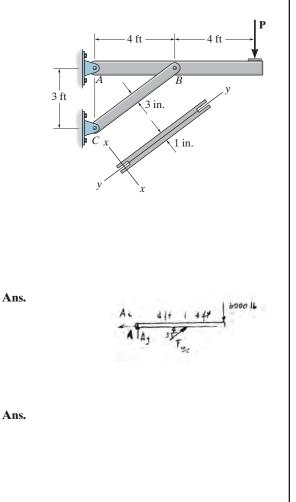
**13–30.** Determine the greatest load P the frame will support without causing the A-36 steel member BC to buckle. Due to the forked ends on the member, consider the supports at B and C to act as pins for x-x axis buckling and as fixed supports for y-y axis buckling.
