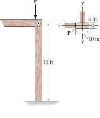
\*13–52. The wood column is fixed at its base and can be assumed fixed connected at its top. Determine the maximum eccentric load *P* that can be applied without causing the column to buckle or yield.  $E_{\rm w} = 1.8(10^3)$  ksi,  $\sigma_Y = 8$  ksi.
