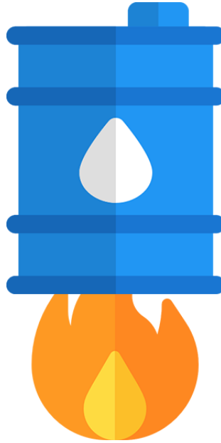
Figure 3.6: If you heat up a sealed barrel the volume of gas cannot increase.
