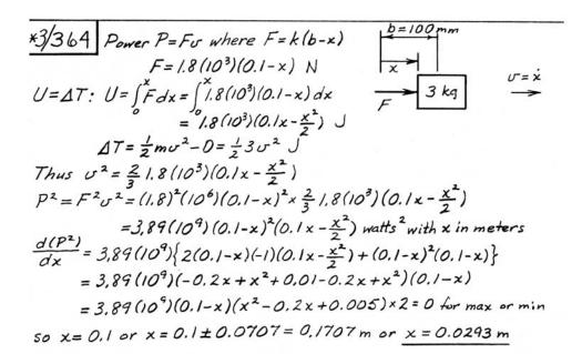
$P = \sqrt{38.9(10^8)} (0.1-x) \sqrt{0.1x - 0.5x^2} W$ Substitute x from above & get  $P_{max} = 220 W$
