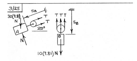
Kinematic constraint:  $L = 2S_A + 3S_B$   $\Rightarrow 0 = 2a_A + 3a_B$  (1)  $\downarrow = \Sigma F = m_A a_A : 30(9.81) \sin 20^\circ - 2T = 30a_A$  (2)  $+ \downarrow = \Sigma F = m_B a_B : 10(9.81) - 3T = 10a_B$  (3) Solution of Eqs. (1)-(3):  $\begin{cases} \frac{a_A = 1.024 \text{ m/s}^2}{a_B = -0.682 \text{ m/s}^2} \\ T = 35.0 \text{ N} \end{cases}$
