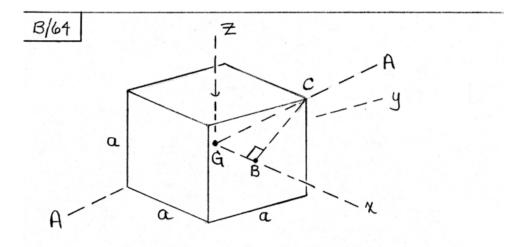
Choose origin of X-y-z axes at center G By Symmetry, the direction cosines of AA are  $l=m=n = \cos \neq BGC$   $\overline{GB} = \frac{a}{2}$ ,  $\overline{BC} = \frac{a\sqrt{2}}{2}$ ,  $\overline{GC} = \frac{a}{2}\sqrt{3}$ , so  $l=m=n=\frac{1}{\sqrt{3}}$   $I_{XX} = I_{YY} = I_{ZZ} = \frac{1}{6}ma^2$ ,  $I_{XY} = I_{XZ} = I_{YZ} = 0$ From Eq. 8/10:  $I_{AA} = 3(\frac{1}{6}ma^2)(\frac{1}{\sqrt{3}})^2$  $= \frac{ma^2}{6}$
