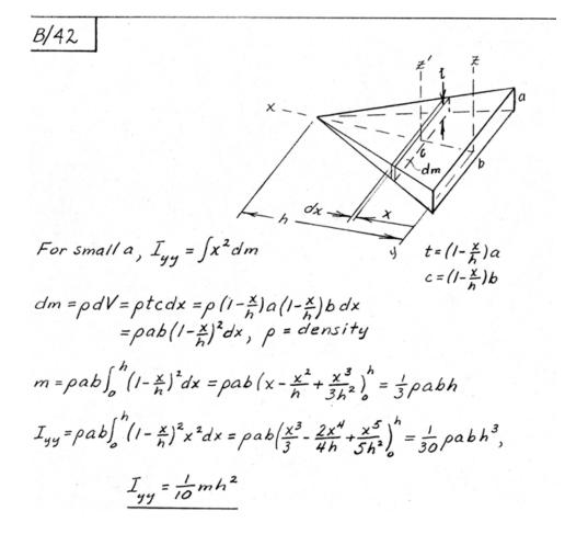
$\frac{B/43}{From the figure in the solution for Prob. B/42 & the ex$  $pression for dm, <math>pab(1-\frac{x}{h})^2 dx$ , the moment of inertia of dm about the z-axis is  $dI_{zz} = dI_{z'z'} + x^2 dm$  by the transfer-of-axis theorem. Also, from the results of Prob. B/42 or Table D/4  $dI_{z'z'} = \frac{1}{12} dmc^2 = \frac{1}{12} dm(1-\frac{x}{h})^2 b^2$
