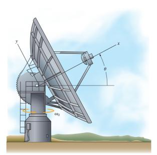
**Problem 20.12** The vertical shaft supporting the disk antenna is rotating with a constant angular velocity  $\omega_0 = 0.2$  rad/s. The angle  $\theta$  from the horizontal to the antenna's axis is 30° at the instant shown and is increasing at a constant rate of 15° per second. The secondary *xyz* coordinate system shown is fixed with respect to the dish.
