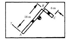
**Problem 20.91** Suppose that the crane described in Example 20.8 undergoes a rigid-body rotation about the vertical axis at 0.1 rad/s in the counterclockwise direction when viewed from above.
