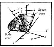
**Problem 20.73** A satellite can be modeled as an 800-kg cylinder 4 m in length and 2 m in diameter. If the nutation angle is  $\theta = 20^{\circ}$  and the spin rate  $\dot{\phi}$  is one revolution per second, what is the satellite's precession rate  $\dot{\psi}$  in revolutions per second?
