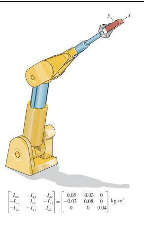
**Problem 20.29** A robotic manipulator holds a casting. The inertia matrix of the casting in terms of a body-fixed coordinate system with its origin at the center of mass is shown. At the present instant, the casting is stationary. If the manipulator exerts a moment  $\Sigma \mathbf{M} = 0.042\mathbf{i} + 0.036\mathbf{j} + 0.066\mathbf{k}$  (N-m) about the center of mass, what is the angular acceleration of the casting at that instant?
